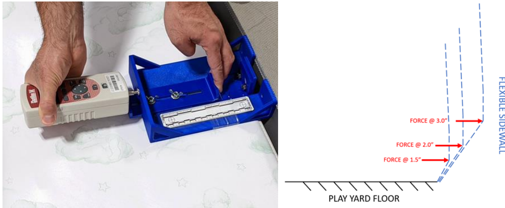
Figure 3. Force application using CPSC's proposed sliding gauge to measure the gap between the mattress and sidewall (left); gap becomes larger with force applied higher above play yard floor (right)
