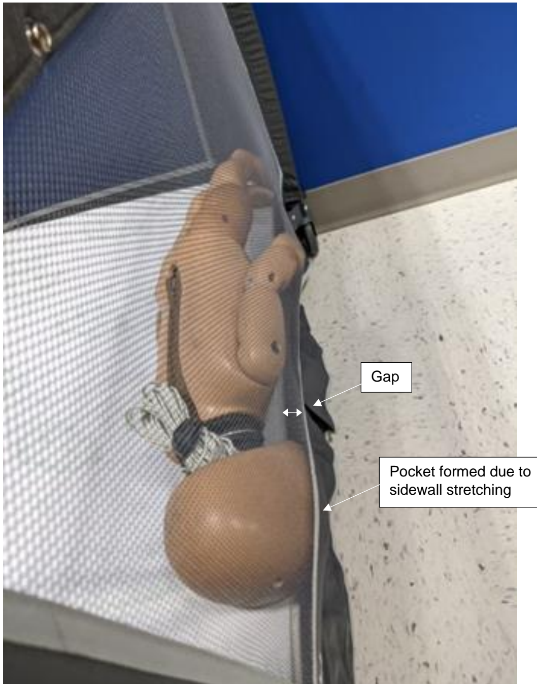
Figure 1. CRABI dummy positioned against the sidewall increases the gap between the mattress and sidewall.
