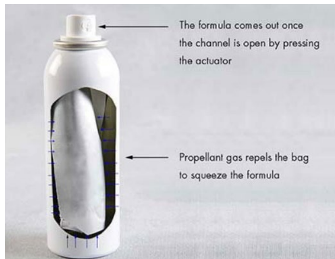
Figure 10: Visual of a BOV system.
