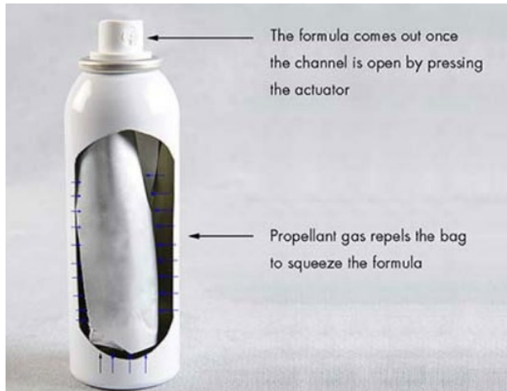
Figure 13: Visual of a BOV system.
