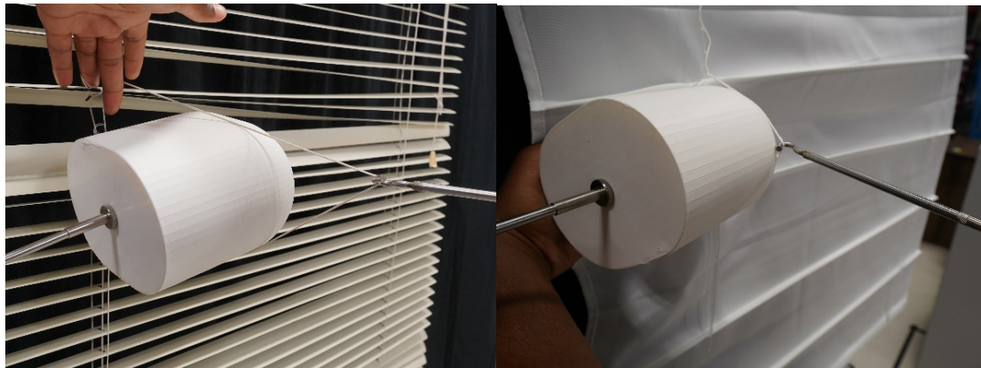
Figure 16. Inserting of the head probe into the inner cord loop and non-rigid cord shroud
