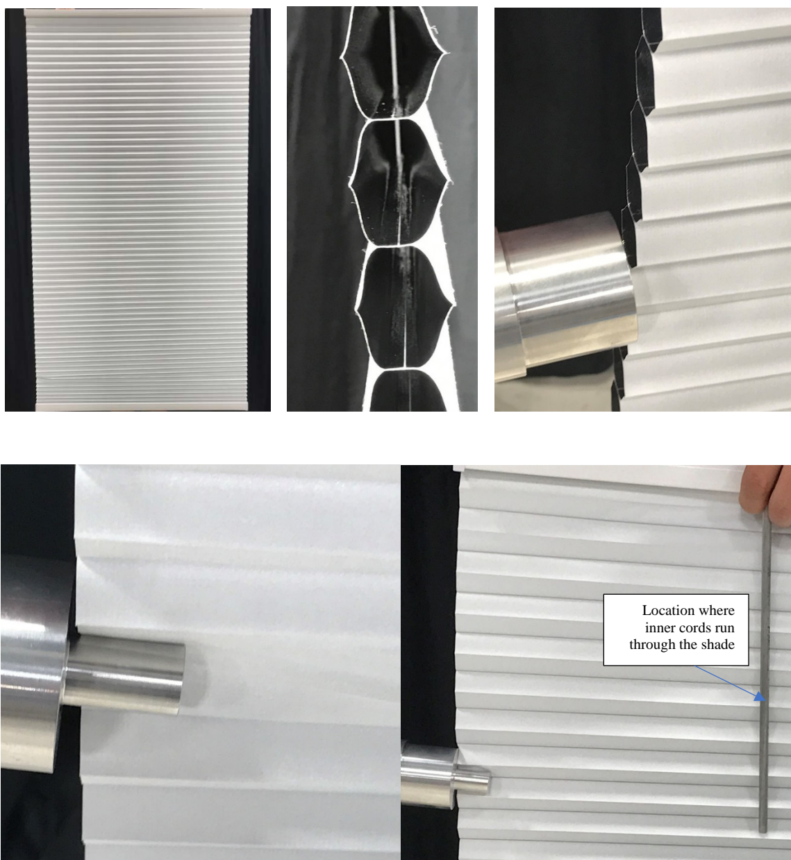
Figure 12. Accessibility to the inner cord in a closed construction (cellular)
