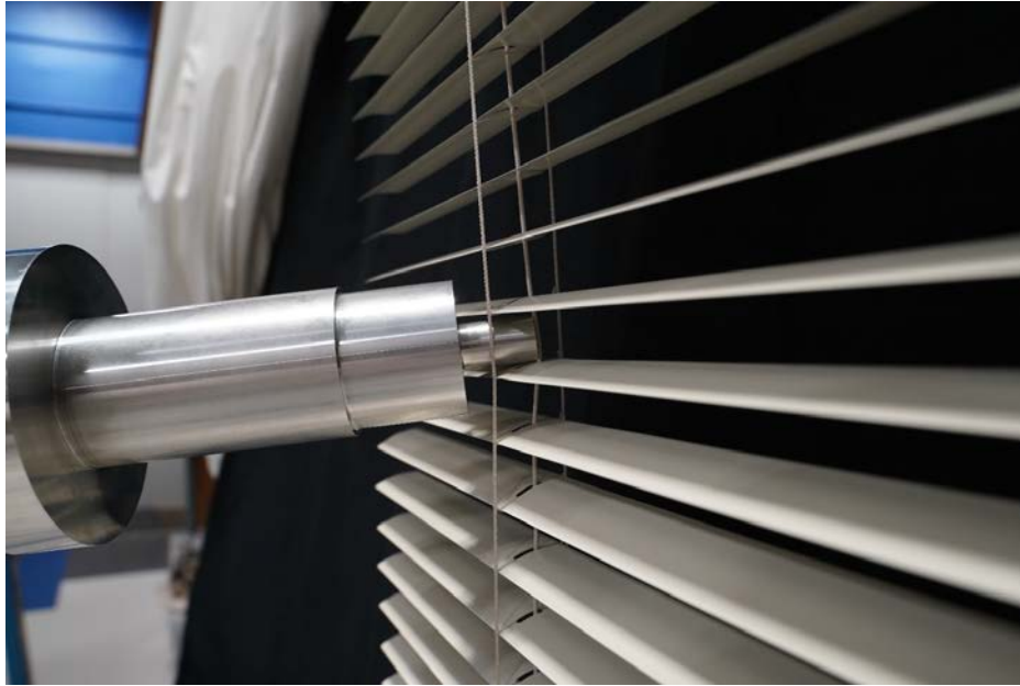
Figure 9. Accessibility to inner cord in an open construction (horizontal)
