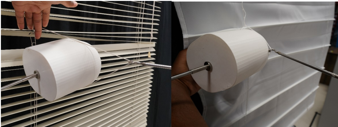
Figure 20. Inserting the head probe into the inner cord loop and nonrigid cord shroud
