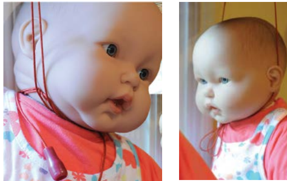
Figure 2. Demonstration of wrapped cords around (doll) child's neck (left), (doll) child's head is through the loop created by entangled multiple cords (right)
