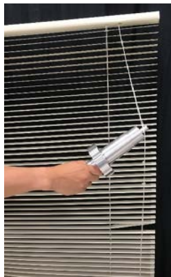
Figure 11a Horizontal Blind with Accessible Operating Cord Using Cord Accessibility Probe
