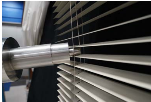
Figure 14. Accessibility to inner cord in an open-construction horizontal blind
