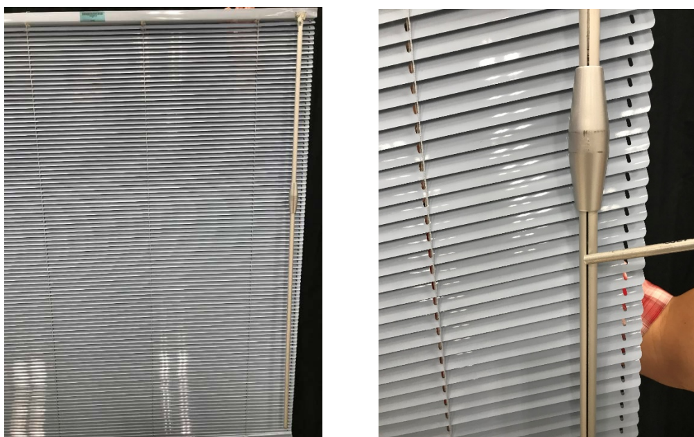
Figure 8. Product with a rigid cord shroud that encapsulates the cord. The cord shroud accessibility probe cannot touch the shrouded cord.
