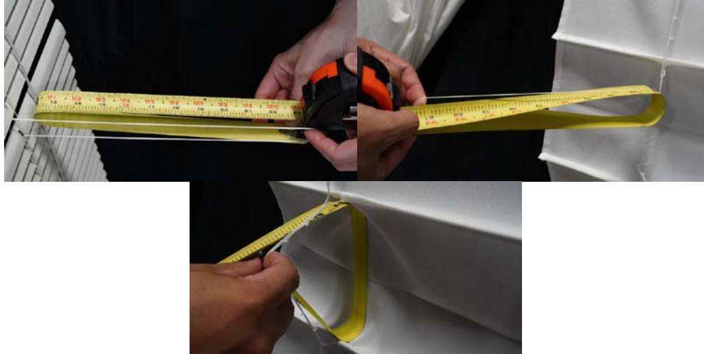
Figure 21. Perimeter measurement on a horizontal blind (top), Roman shade inner cord (middle), and Roman shade inner cord shroud (bottom)
