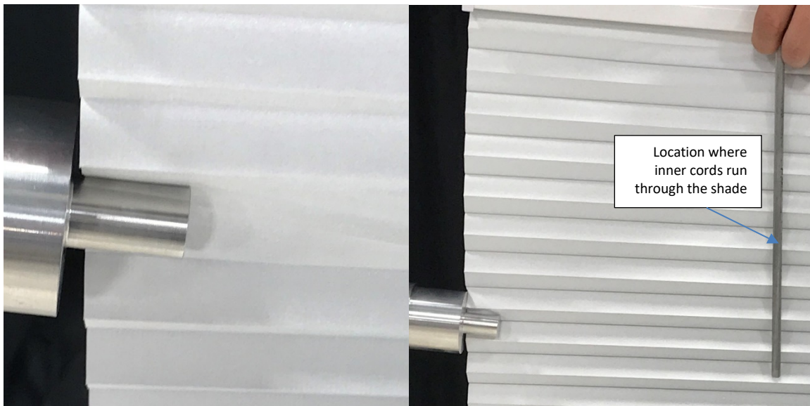
Figure 16. Accessibility to the inner cord in a closed construction (cellular) window covering
