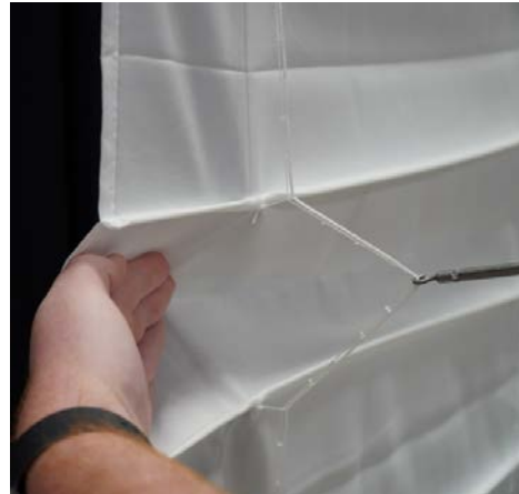
Figure 19. Nonrigid shroud opening on a Roman shade
