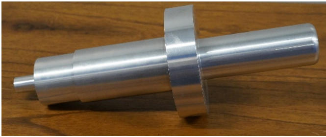
Figure 1. Cord Accessibility Probe
