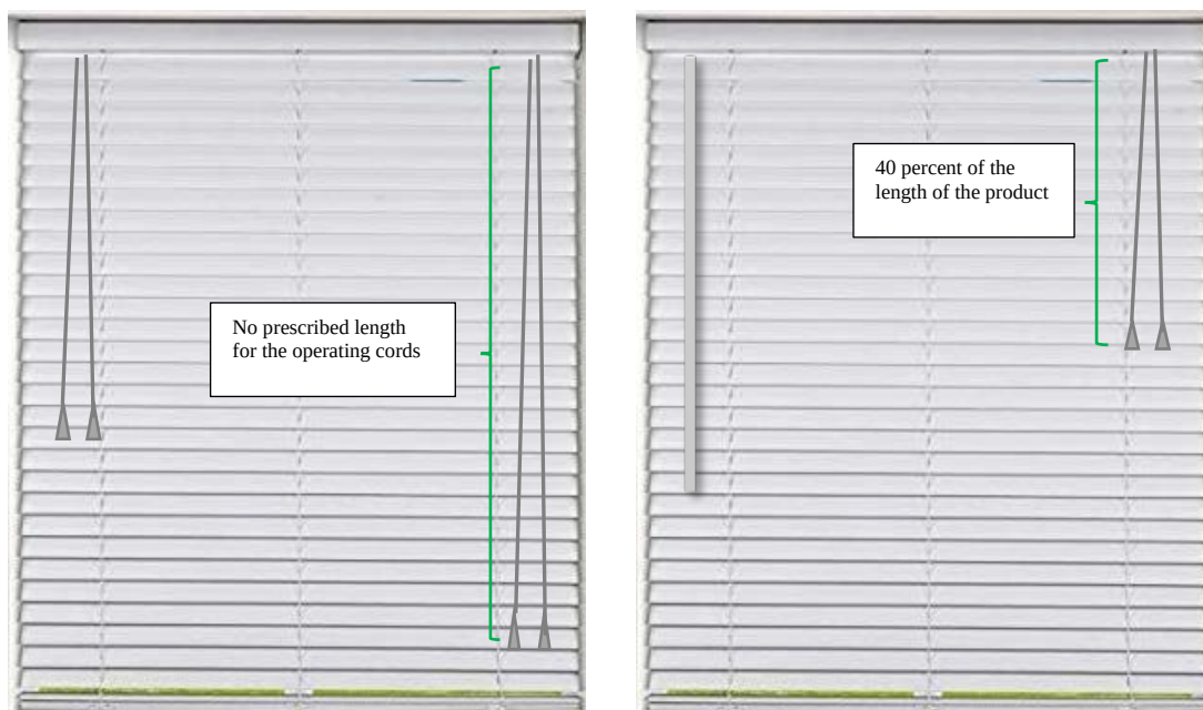
Figure 1. Window blind with operating cords longer than 40 percent of the length of the product and tilt cords to tilt the slats (left). Window blind with operating cords equal to 40 percent of the product length and wand tilt replacing tilt cords (right)
