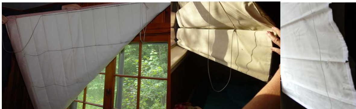
Figure 7. Accessible and hazardous inner cords from IDIs 090728CCC2792 (left), 110607CCC3794 (middle), 140305CBB1435 (right)
