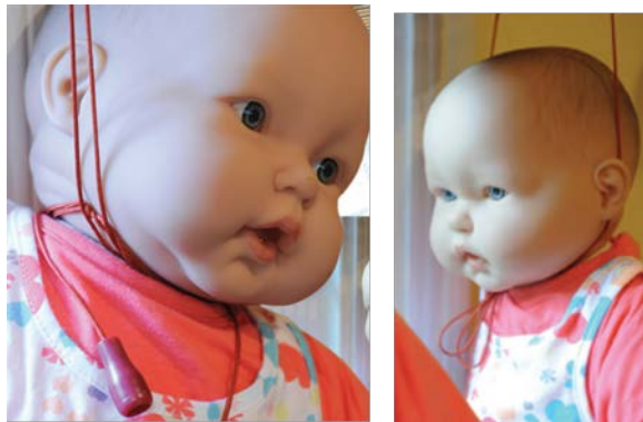
Figure 17. Demonstration of wrapped cords around (doll) child's neck (left), (doll) child's head is through the loop created by entangled multiple cords (right)
