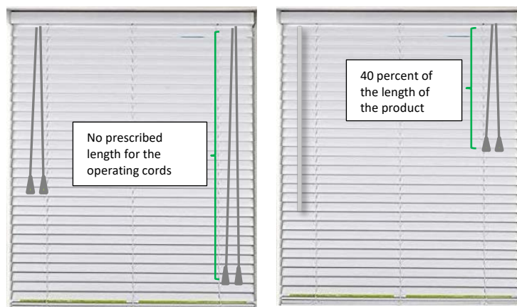
Figure 16. Window blind with operating cords longer than 40 percent of the length of the product and tilt cords to tilt the slats (left). Window blind with operating cords equal to 40 percent of the product length and wand tilt replacing tilt cords (right)
