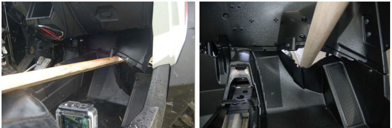
Figure 4 – Comparison of Full-Scale Robotic ROV Test and Sled Test; Left – Robotic ROV Test Where Dowel Penetrated the Seam that Joins the Floorboard and Firewall Panels; Right – Sled Test Where the Dowel Penetrated the Seam that Joins the Floorboard and Firewall Panels
