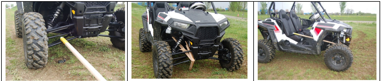
Figure 3 – Multiple Views of the Robotic ROV; Left – Alignment of the Test Dowel with Test Target on the ROV Floorboard; Middle – Front View of Broken Dowel After Collision at 10 mph; Right – Side View of Test Dowel that Entered the ROV Passenger Occupant Area
