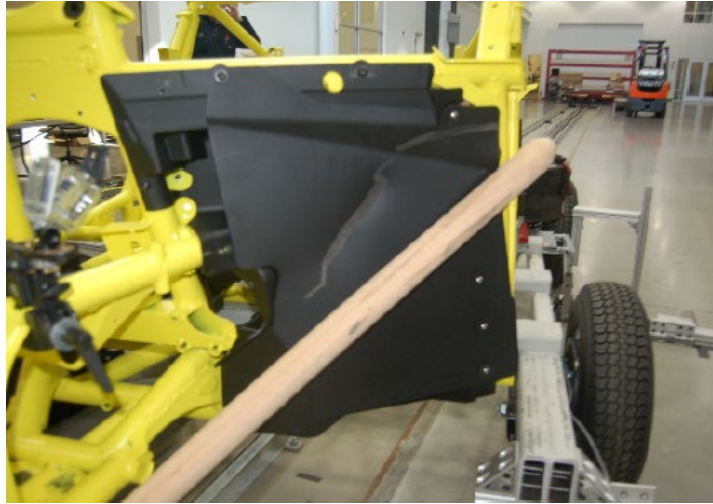
Figure 6 – Illustration of an Aluminum Floorboard Guard that Redirected the Test Dowel and Prevented Debris Penetration (at 5 mph)
