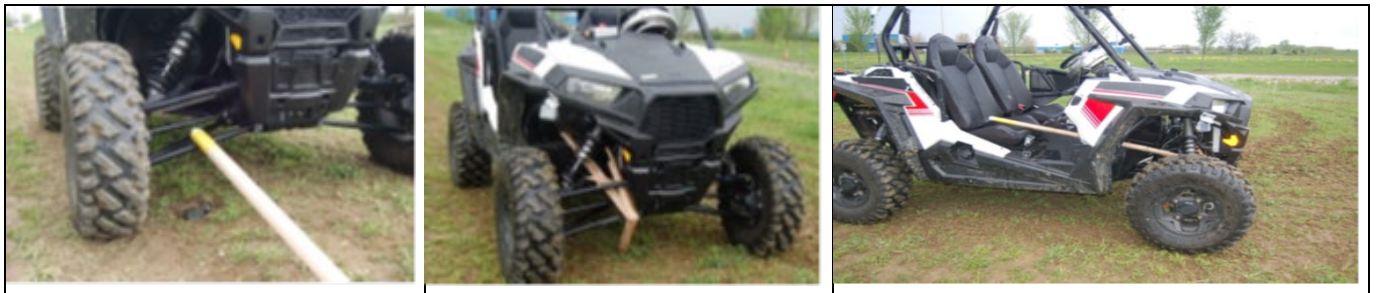
Figure 2 – Multiple Views of the Robotic ROV involving Collision at 10 mph; Left – Alignment of the Test Dowel with Test Target on the ROV Floorboard; Middle – Front View of Broken Dowel; Right – Side View of Test Dowel that Entered the ROV Passenger Occupant Area
