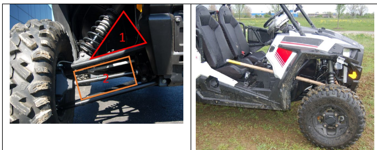
Figure 5 – Illustration of Wheel Well Target Zones (Left); Dowel Penetration Where the Dowel Passed Through Zone 2 Control Arm Components (Right)
