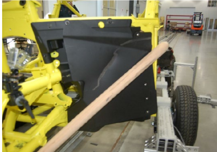
Figure 7 – Illustration of an Aluminum Floorboard Guard that Redirected the Test Dowel and Prevented Debris Penetration (at 5 mph)
