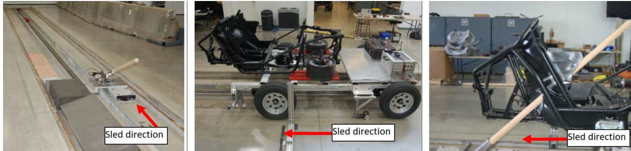
Figure 3 – Multiple Views of the Simulated Vehicle Test Sled; Left – Test Dowel in Relation to the Direction of the Test Sled; Middle – Side View of an Example of a Fully Loaded Test Sled; Right – Side View of a Sled Test Where the Test Dowel Penetrated the ROV Floorboard
