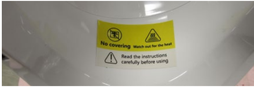
Figure 8. Non-compliant with UL 1278, section 67.14 warning label.
