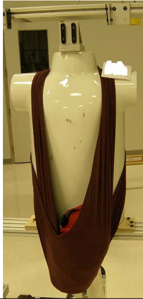
Figure 1: Test mass is not supported in a proper position at the beginning of the test. Test mass ejected.
