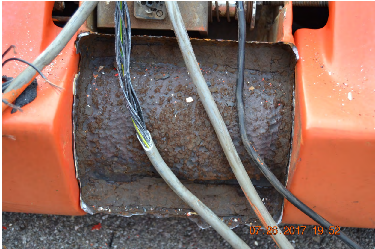
Photo #15 – Additional close up picture of the incident ride. Photo identifies the inside of the arm on the gondola that separated from the ride. Photograph taken by the [REDACTED] State Highway Patrol on July 26, 2017 after the incident.
