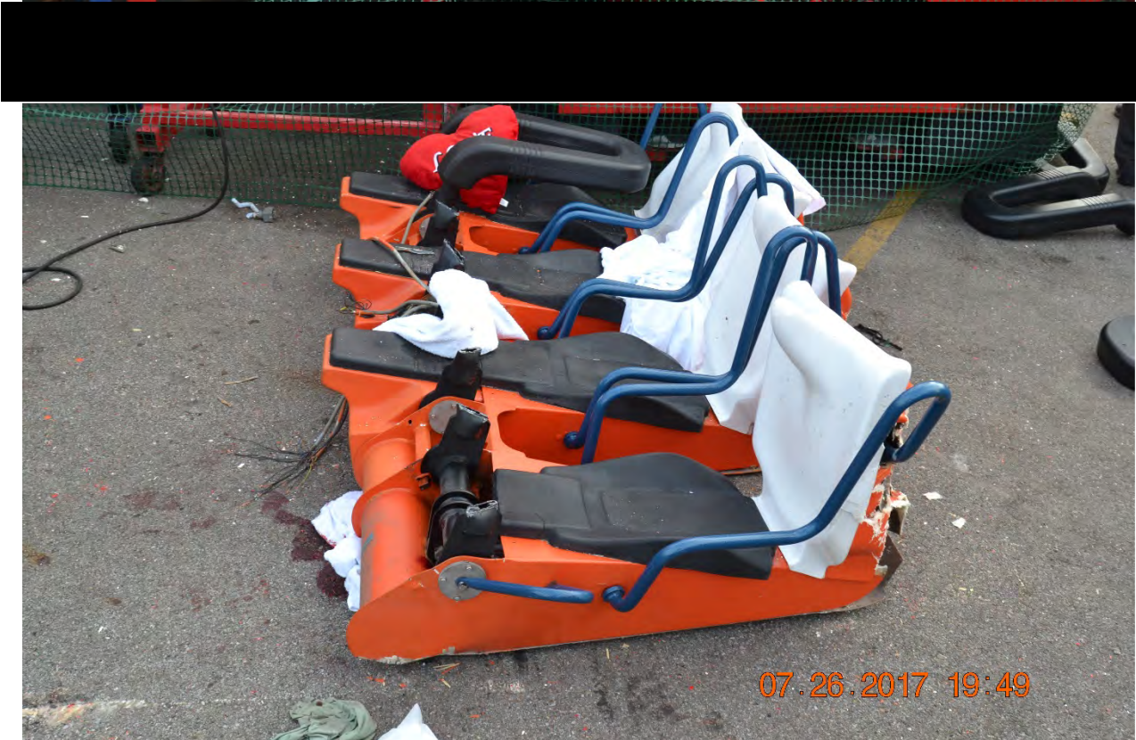
Photo #11 – Additional close up picture of the incident ride. Photo identifies the gondola that separated from the ride. Photograph taken by the [REDACTED] State Highway Patrol on July 26, 2017 after the incident.
