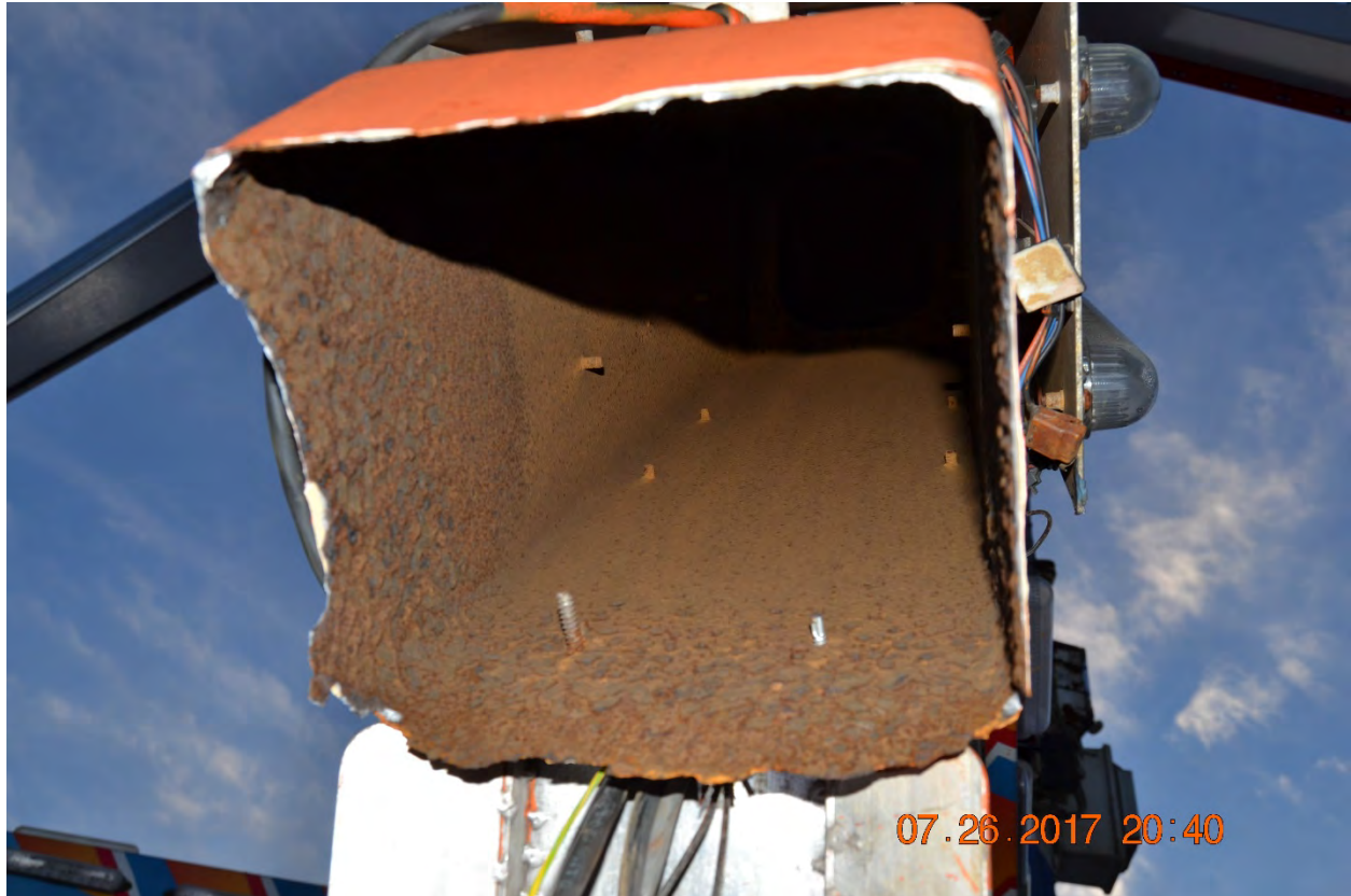
Photo #21 – Additional close up picture of the incident ride. Photo identifies the inside of the wall of metal around the arm of the broken gondola. Photograph taken by the [REDACTED] State Highway Patrol on July 26, 2017 after the incident.
