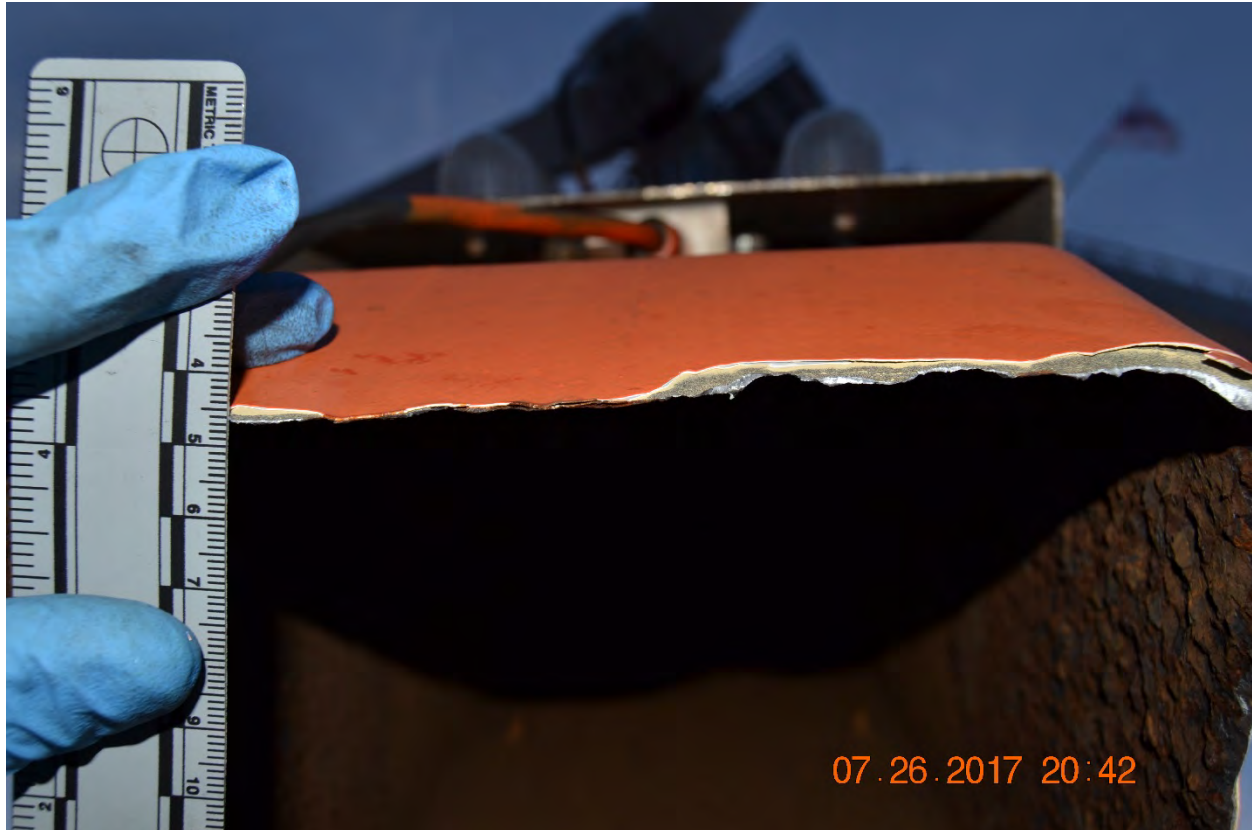
Photo #23 – Additional close up picture of the incident ride. Photo identifies the inside of the wall of metal around the arm of the broken gondola. Photograph taken by the [REDACTED] State Highway Patrol on July 26, 2017 after the incident.
