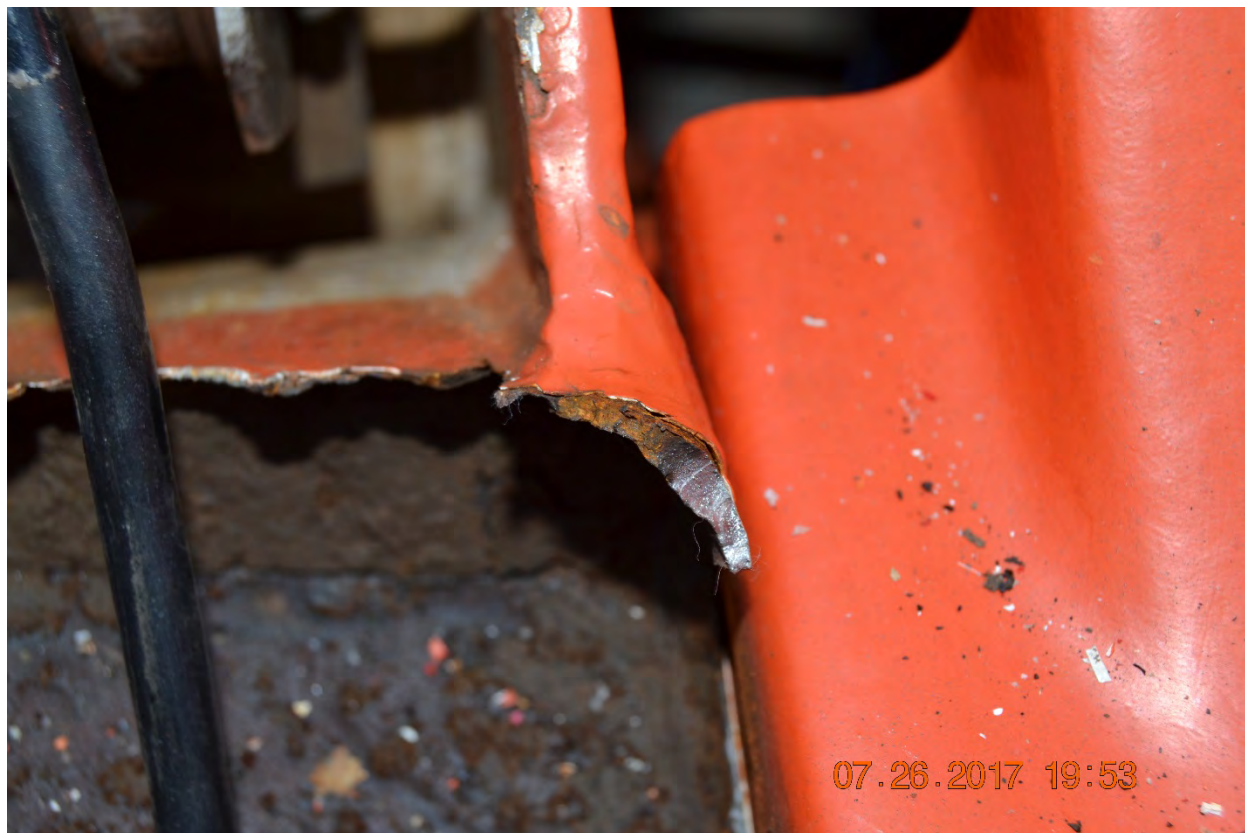
Photo #16 – Additional close up picture of the incident ride. Photo identifies the inside of the arm on the gondola that separated from the ride. Photograph taken by the [REDACTED] State Highway Patrol on July 26, 2017 after the incident.
