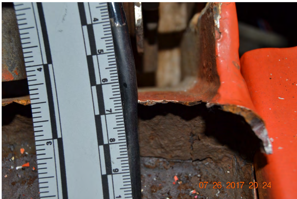
Photo #19 – Additional close up picture of the incident ride. Photo identifies the wall of metal around the arm of the broken gondola. Photograph taken by the [REDACTED] State Highway Patrol on July 26, 2017 after the incident.
