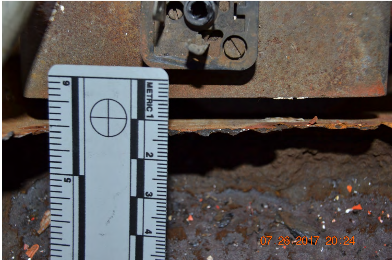
Photo #20 – Additional close up picture of the incident ride. Photo identifies the wall of metal around the arm of the broken gondola. Photograph taken by the [REDACTED] State Highway Patrol on July 26, 2017 after the incident.
