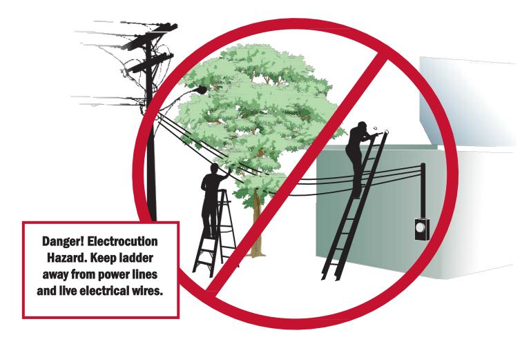
Despite these and other warnings, electrocutions still occur each year. To avoid this hazard, CPSC advises you to use a ladder that does not conduct electricity, such as fiberglass with non-conductive side rails when working near overhead wires. Non-conductive ladders should be kept clean to maintain their non-conductive safety properties.
