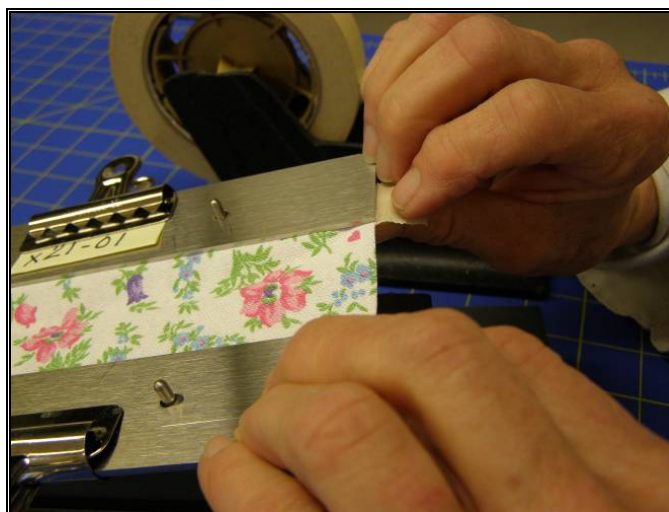
Figure 9. Tape may be used to further secure specimen.
