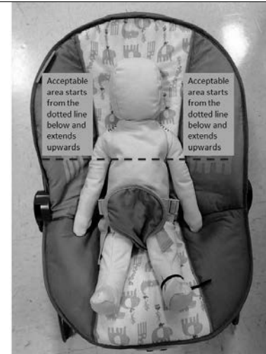
Fig 10. Allowable area for warning label placement starts from the dotted line that crosses the junctions of underarm and both sides of the torso.
