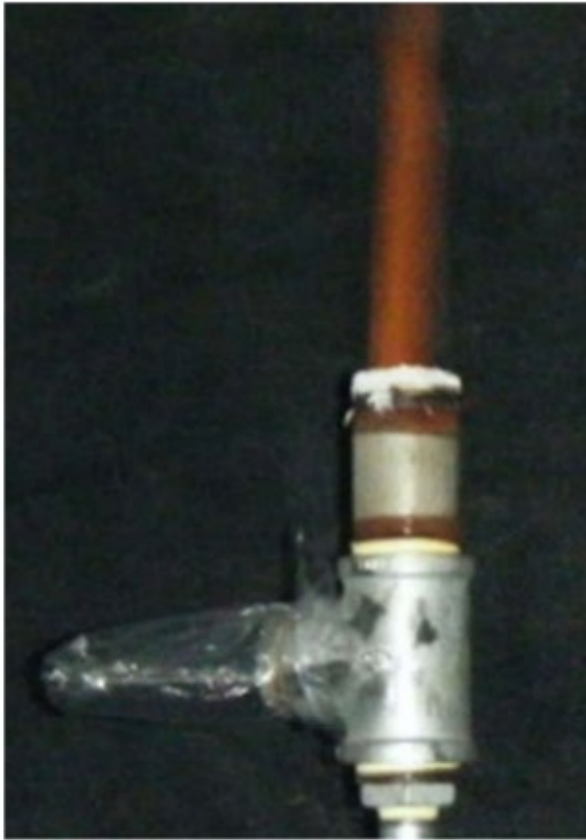
Figure 6 - UL 30 Flame Arrester Test picture (From ANSI/CAN/UL/ULC 30:2022, Standard for Safety Metallic and Nonmetallic Safety Cans for Flammable and Combustible Liquids, Figure 18.4 Example of Correct Stoichiometric Flame. Copyright ULS Inc. 2022).
