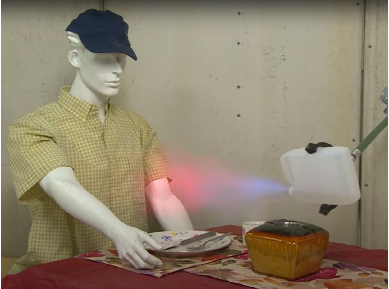
Figure 1- Image from CPSC video demonstrating the hazard of flame jetting with gelled alcohol fuels, 2011.
