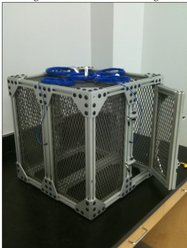
Figure 2: Constructed Blast Cage
