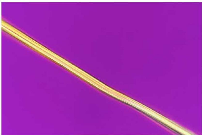
FIGURE 18-B: TICKING FILL FIBERS, YELLOW IN THE NORTH-WEST TO SOUTH-EAST DIRECTION, 400X
