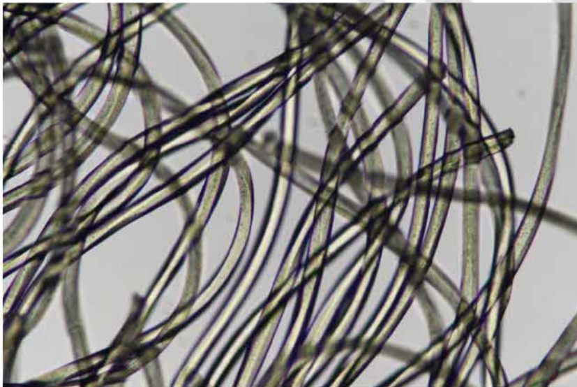
FIGURE 3-B: INNER SURFACE TICKING FIBERS, 400X
