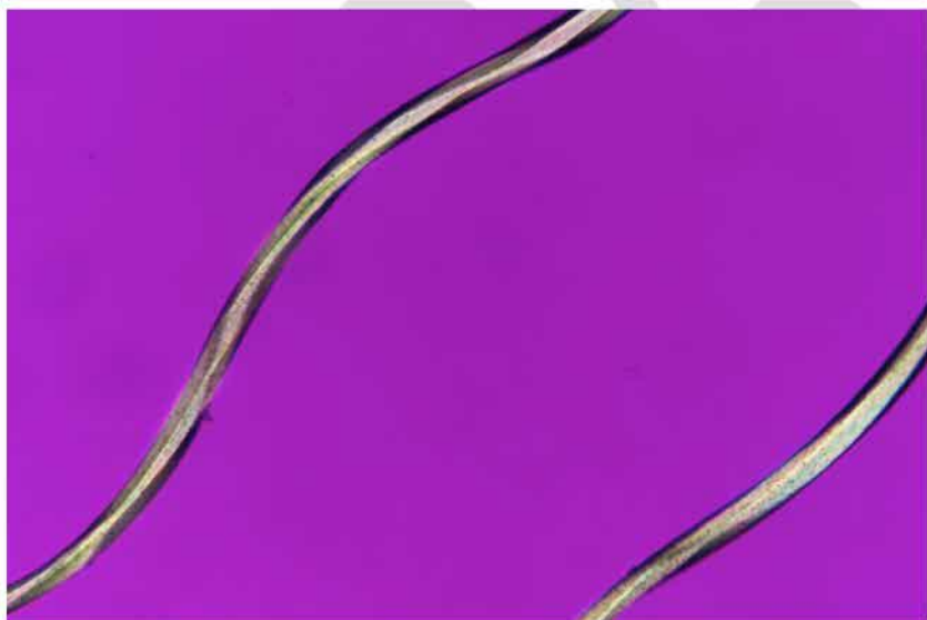
FIGURE 6-A: TICKING FILL FIBERS, LIGHT YELLOW IN THE NORTH-EAST TO SOUTH-WEST DIRECTION, 400X
