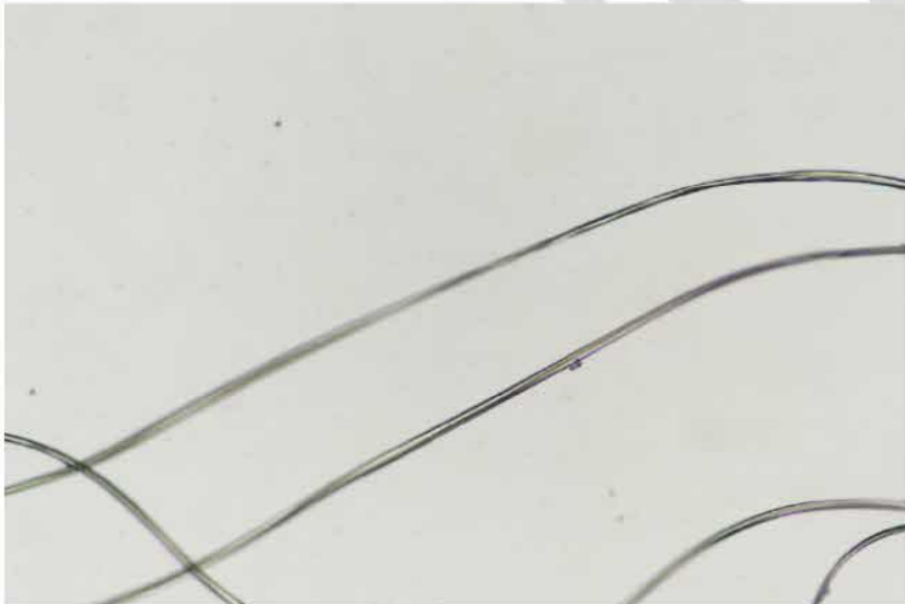
Ticking Inner surface fibers 100x
