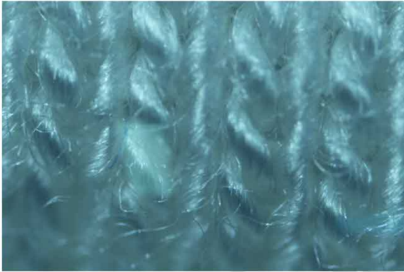
Figure 11-A: Ticking Outer Surface, 40x
