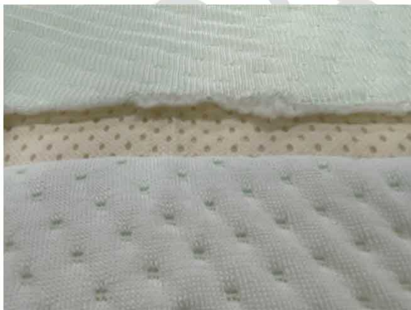
FIGURE 1-B: TICKING, CLOSE UP OF OUTER SURFACE (WHITE), INNER SURFACE (MINT) AND FILL FIBERS
