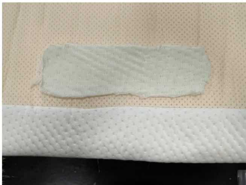
FIGURE 1-A: TICKING, OUTER SURFACE (WHITE), INNER SURFACE (MINT) AND FILL FIBERS
