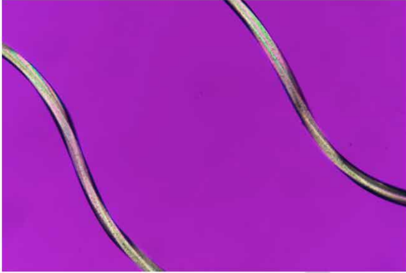
FIGURE 6-B: TICKING FILL FIBERS, LIGHT BLUE IN THE NORTH-WEST TO SOUTH-EAST DIRECTION, 400x
