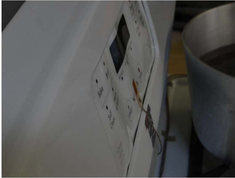
Figure 12-1 Warping of Touch Panel Membrane for Brand A Gas Range during Testing
