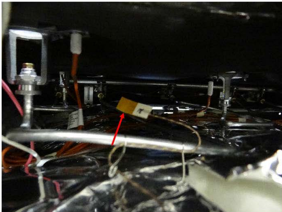
Figure 8-4 Example of Thermocouple Oven Insulation Location/Brand C Test Sample
