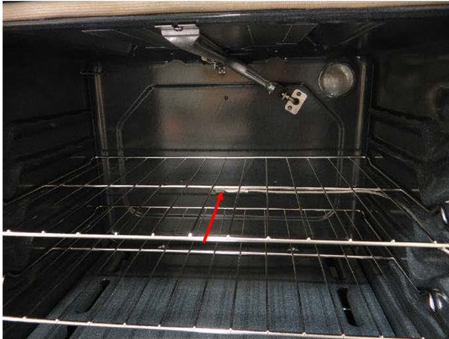
Figure 8-3 Example of Thermocouple Oven Cavity Location/Brand B Test Sample
