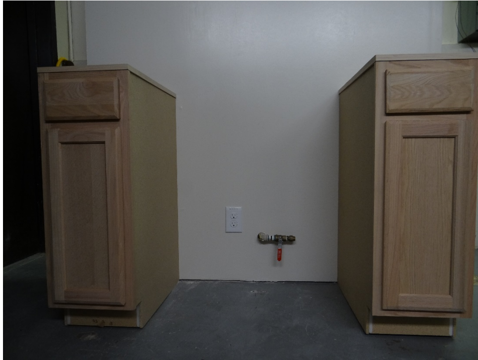
Figure 10-5 Gas Supply and Electrical Outlet Location for Gas Range Test Samples
