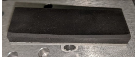
Tapered wear of Slider 55 chamfer due to chatter
