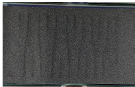
Chatter marks on P400 sandpaper used for Slider 55 conditioning
