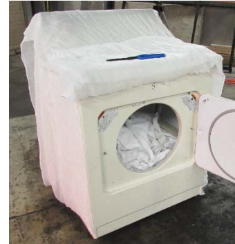
Figure 1. Clothes dryer being prepared for the fire containment test
