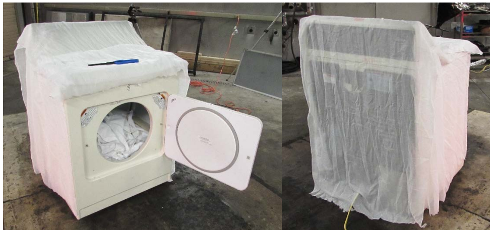
Shown with the door open; door was closed and covered with cheesecloth during the test (not final test set-up)
