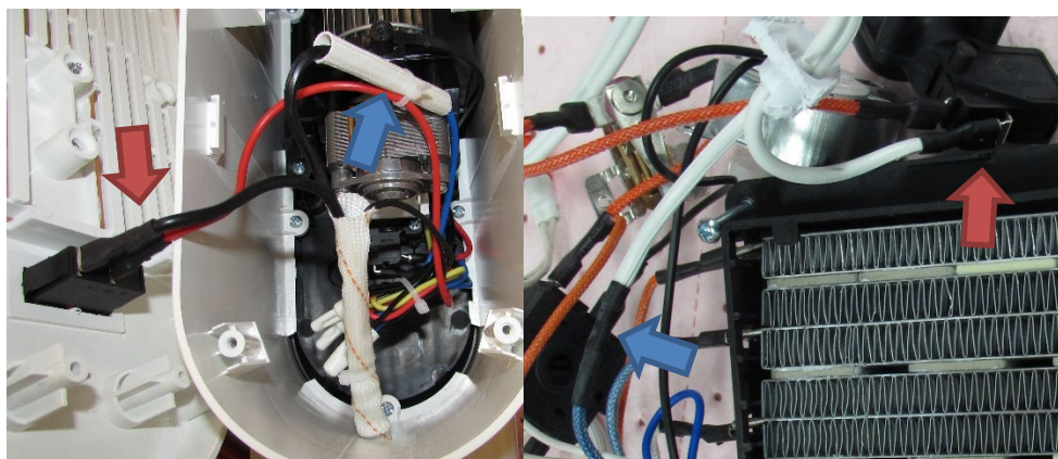
(b) One conductor connected to power switch and other connected to internal wire
