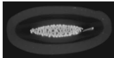
(b) Cross section of butt connector
