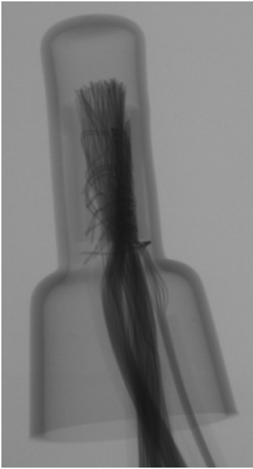
(a) X-ray image of butt connection
