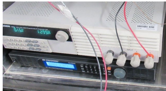
Power supply and load bank
