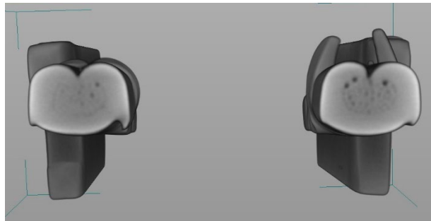
S9 – Cross section of crimps
