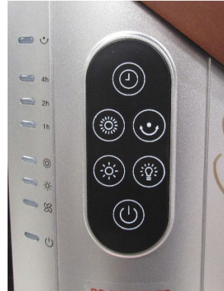
Digital heat selector switch (S2)
