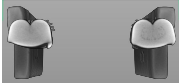
S23 – Cross section of crimps
