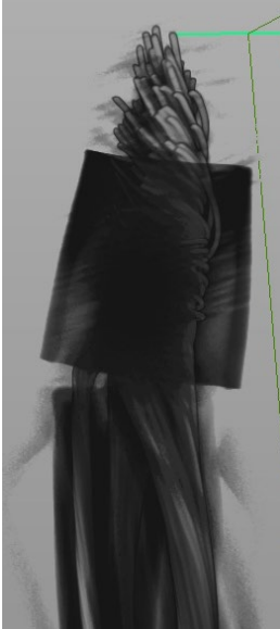
(a) CT image of butt connection
