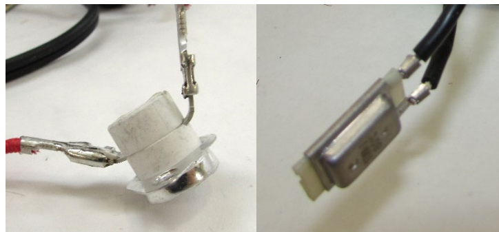
Automatic-reset High Limit Devices
