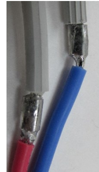
(f) Barrel crimp connection
