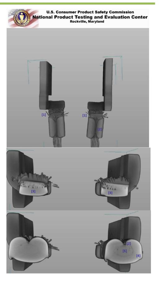
This is an exemplar sample. Crimp and weld configuration.
