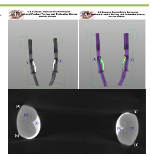
This is an exemplar sample. Crimp and weld configuration.
