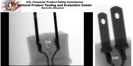
This is an exemplar sample. Crimp and weld configuration. (Note: Black box added to conceal manufacturer markings)
