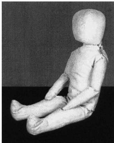
FIG. 2 CAMI Newborn Dummy (7.5 lb., 3.4 kg)
