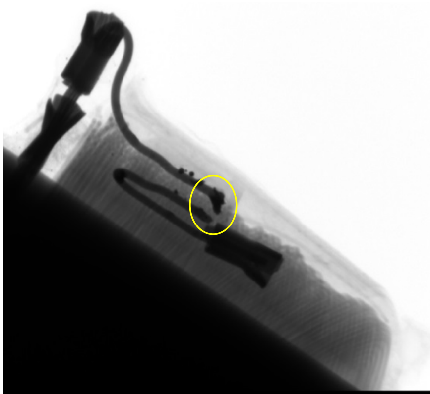
Figure 42. Radiograph of the TCO after the test (sub 73)
