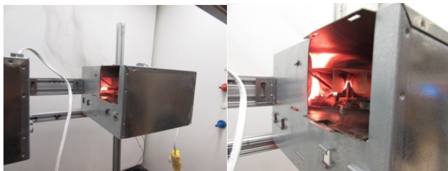
Figure 19. Bypassed TCO lock-rotor test
