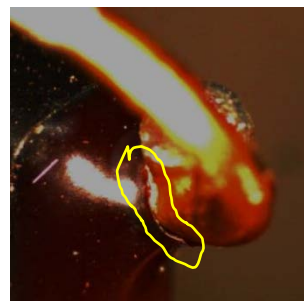
Solder in the cracks of the epoxy/electrode
