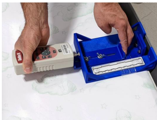
Figure 2. Gap measurement sliding gauge with 5 lbf. applied to main gauge body towards play yard sidewall, and resulting gap measured in the loaded, static position. The raised center section of the gauge is held in place while the force is applied.
