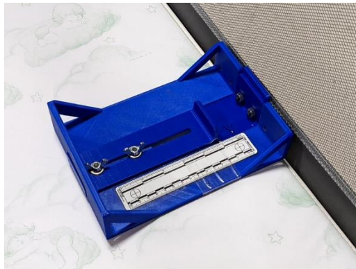
Figure Y. Gap measurement sliding gauge positioned with vertical flanges between edge of mattress and play yard sidewall.
