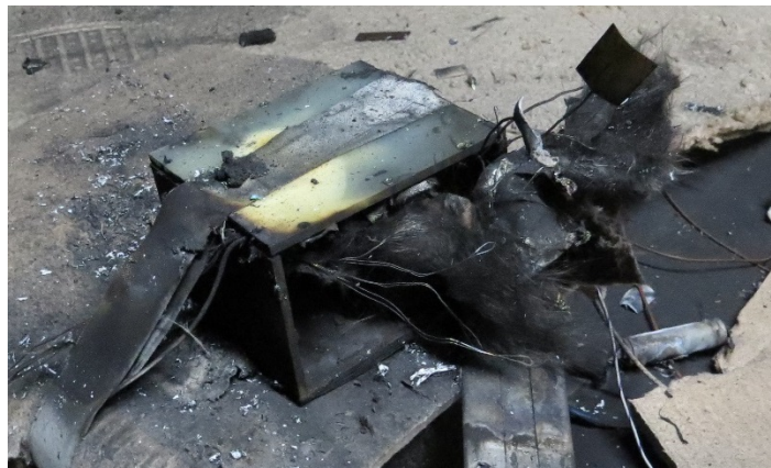
Figure 44. Digital photograph of Pack E3 following propagating thermal runaway
