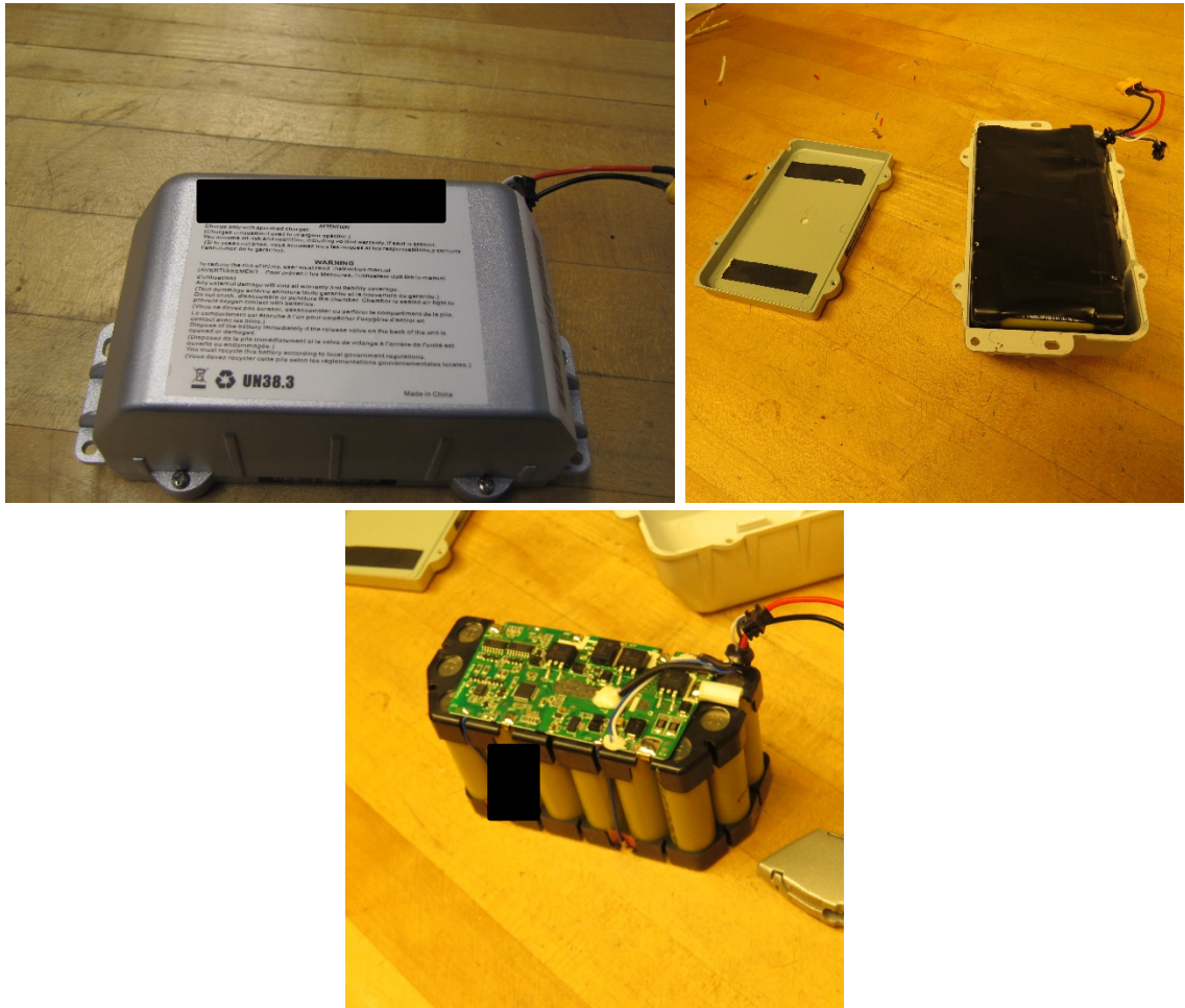
Figure 3. Pack B, comprised of twenty Li-Ion ICR18650 cells in a 10S2P configuration
