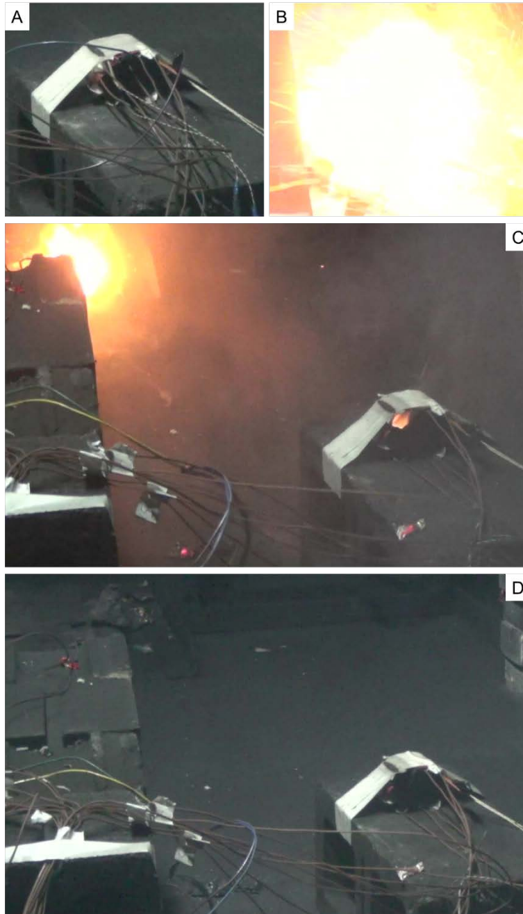
Figure 35. Video screenshots from Pack D2 immediately prior to trigger cell failure (A), energetic failure of trigger cell resulting in sparks and flame (B), ejection of cell contents from trigger cell (C), remaining cells intact after trigger cell ejection (D)
