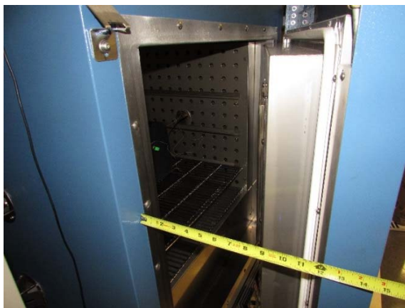
Figure 4.6. Oven chamber door partially opened about 9 inches (23 cm)
