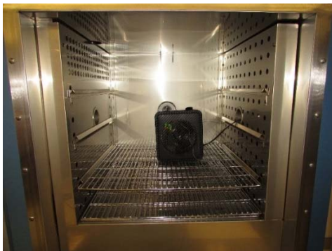
Figure 4.3. Heater inside the conditioning oven
