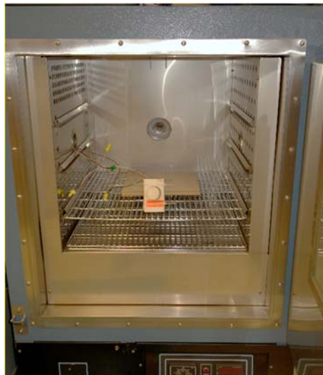
Figure 4.11. Thermostat in the conditioning oven
