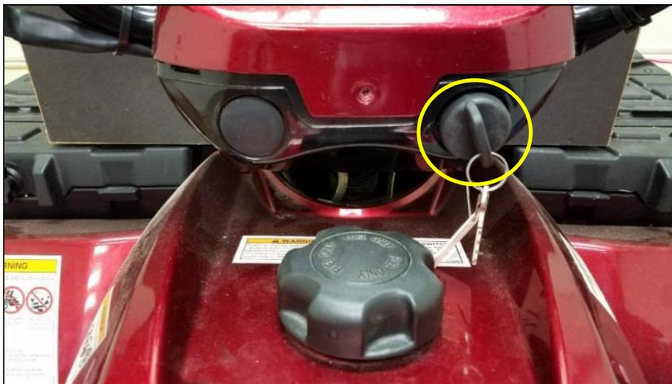
Figure 3-5. Key under center console (activation required for the Standard ignition)
