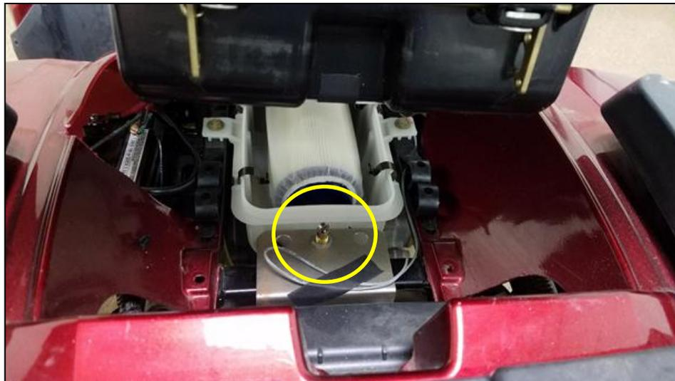
**Figure 3-6.** Pressure switch under rear of seat (activation required for the CR prototype ignition)
