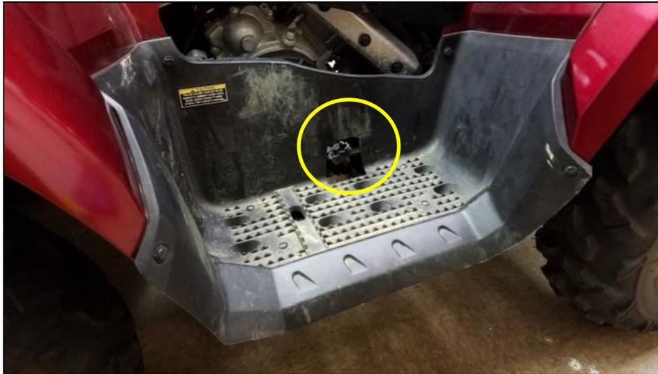
**Figure 3-2.** Foot brake in right foot well (activation required for both the Standard and CR prototype ignitions)
