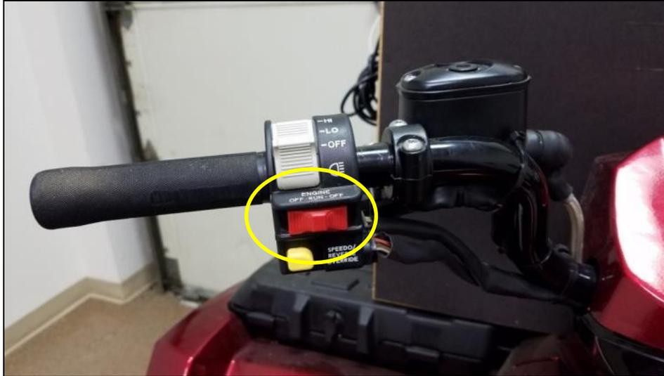
Figure 3-4. Engine Run switch on left handle bar (activation required for both the Standard and CR prototype ignitions)
