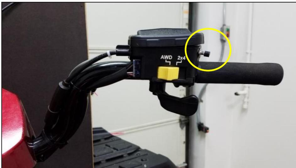
**Figure 3-3.** "Start" button on right handle bar (activation required for the CR prototype ignition)
