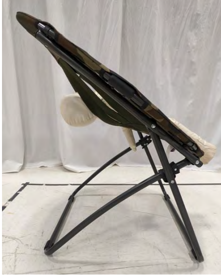
Figure 3. Demonstration of a 6-month CAMI's head entrapped between the elastic components of the seatback.
