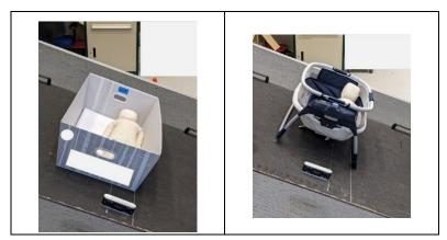
Figure 3. Compact Bassinet/Cradle Tests to 20 deg tilt angle
