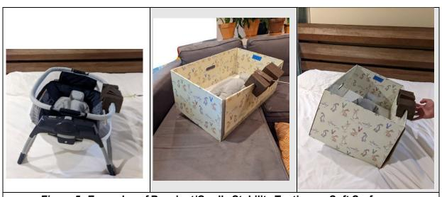
Figure 5. Examples of Bassinet/Cradle Stability Testing on Soft Surfaces
