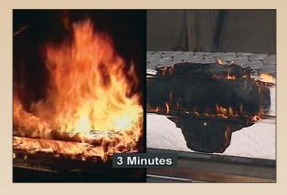
A conventional mattress is in flames in just a few minutes compared to a mattress that complies with the federal open-flame standard, on the right.
