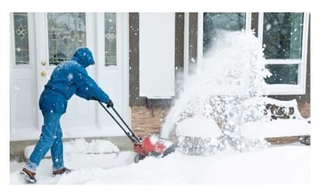
Most snow thrower injuries happen when consumers try to clear snow from the discharge chute or debris from the auger/collectors. Always stop the engine before attempting to clear snow and debris from any part of the snow thrower.
