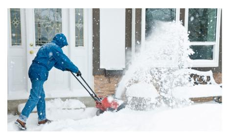
Most snow thrower injuries happen when consumers try to clear snow from the discharge chute or debris from the auger/collectors. Always stop the engine before attempting to clear snow and debris from any part of the snow thrower.
