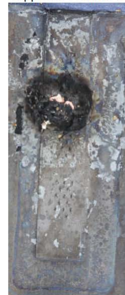
Negative Electrode Opposite Positive Tab
