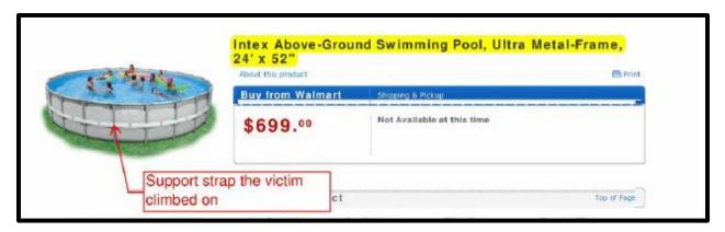
Ladder removed from pool when not in use. Child was a climber, and would use the side support strap as a step. Dirt marks were found on side of pool near the center support strap.
