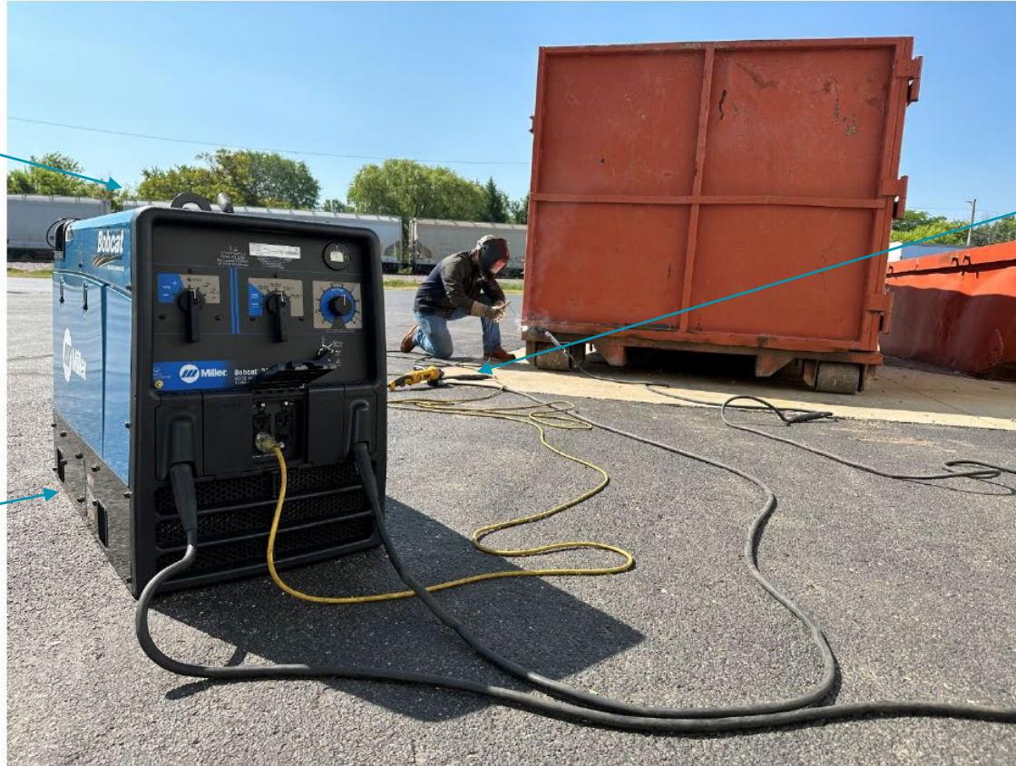
Photo 1: Typical Welding Application with a Grinder Attached with Auxiliary Power
