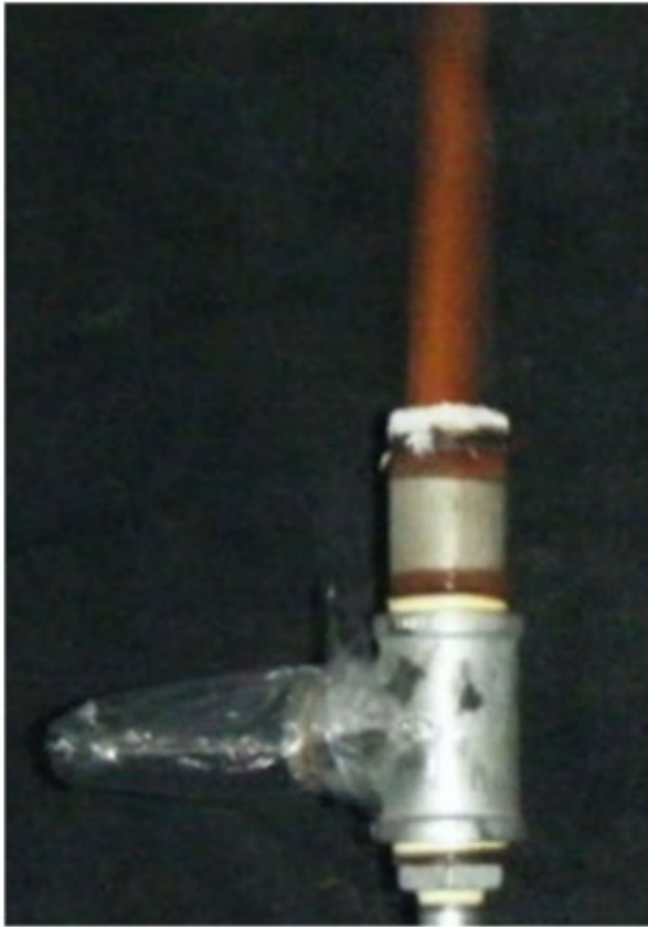
Figure 5 - UL 30 Flame Arrester Test picture (From ANSI/CAN/UL/ULC 30:2022, Standard for Safety Metallic and Nonmetallic Safety Cans for Flammable and Combustible Liquids, Figure 18.4 Example of Correct Stoichiometric Flame. Copyright ULS Inc. 2022).
