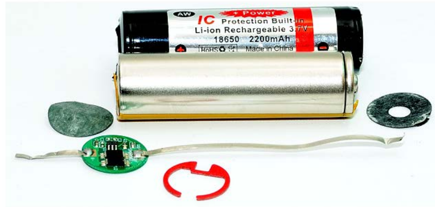
Figure 5. The anatomy of a protected 18650 battery by Lygte Info
