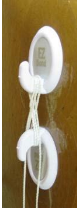
Figure 17. An improvised cleat would serve as the connection point to furniture. In this photo it has been wrapped in a figure-eight to remove the slack from a corded tether.
