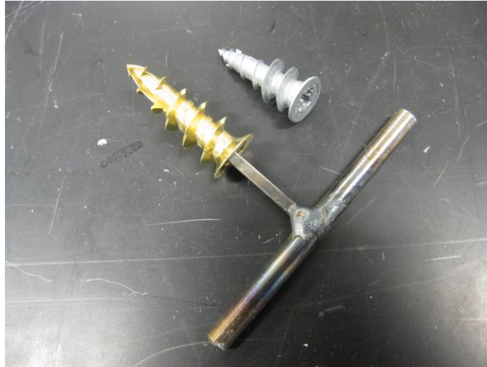
Figure 2. The drywall anchors were able to be inserted with two pieces of readily available metal rods welded together.
