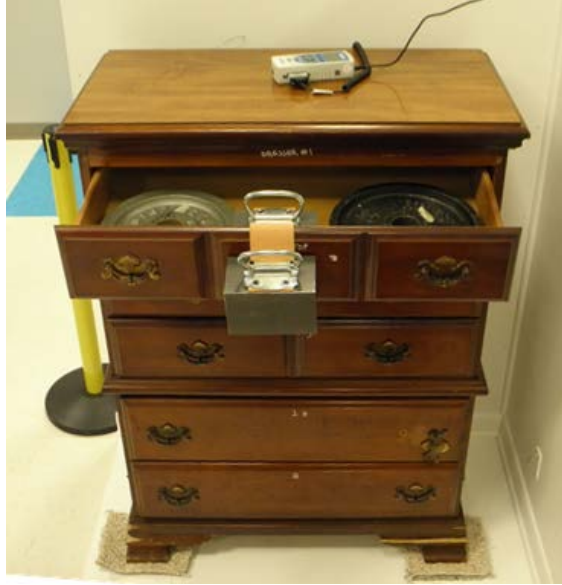
Figure 16. Small squares of carpet and padding were used to simulate a carpeted environment.
