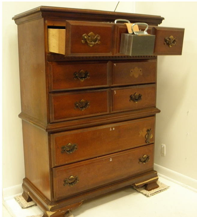
Figure 1. The dresser used to evaluate new tip-restraint ideas is shown here saddled with two 25-lbm steel blocks.
