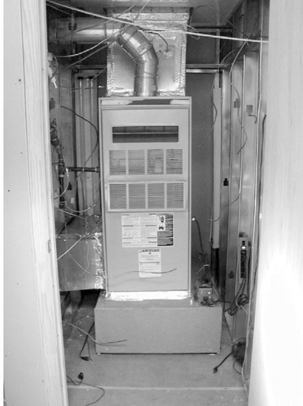
Figure 2.1. Draft Hood Equipped Test Furnace
