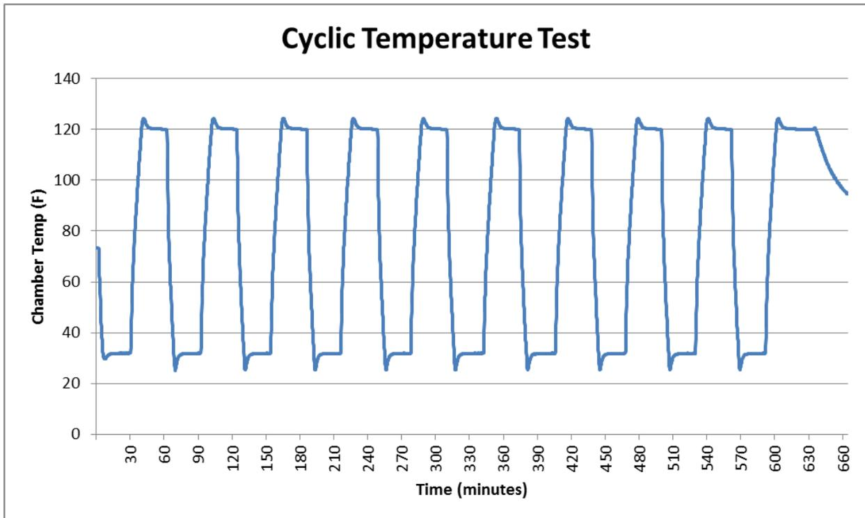
Figure 1. UL 2034 Section 42.1 C Cyclic Temperature Test Temperature Modulation.
