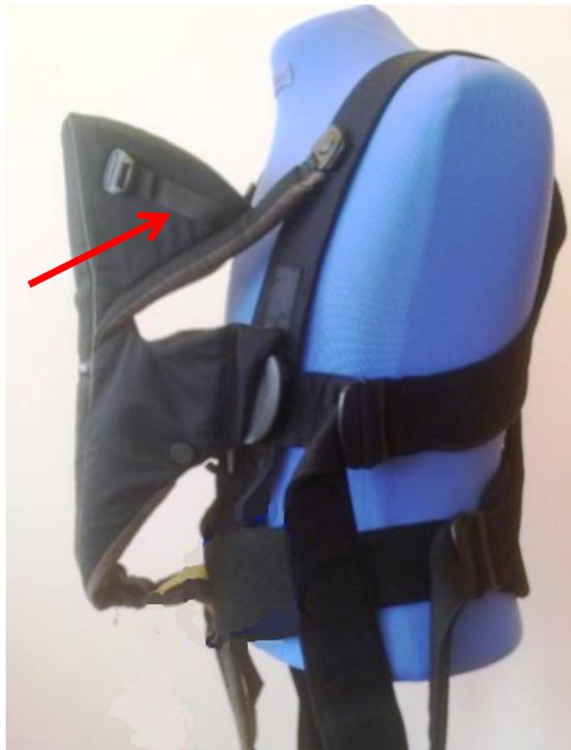
Figure 1. Example of Non-Load-Bearing Head Adjustment Fastener
