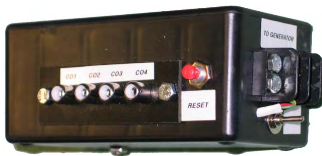
Figure 2: Automatic CO Safety Shutoff Device Control Box
