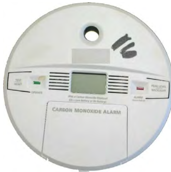
Figure 5: Typical CO Alarm used to measure the CO concentration during generator testing
