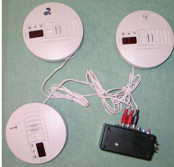
Figure 3: Automatic CO Safety Shutoff Device: Control Box with Three Model 1 CO Alarms Connected
