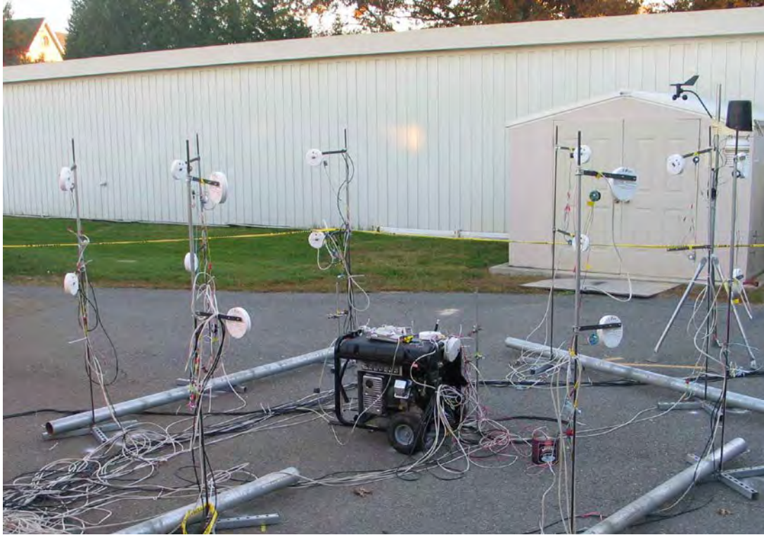
Figure A4: Generator in Courtyard Surrounded by Sensors and CO Alarms
