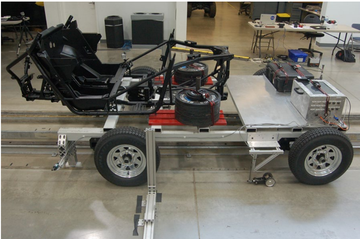
Figure 35: Sled Cart with OEM ROV Frame (Vehicle A) Attached
