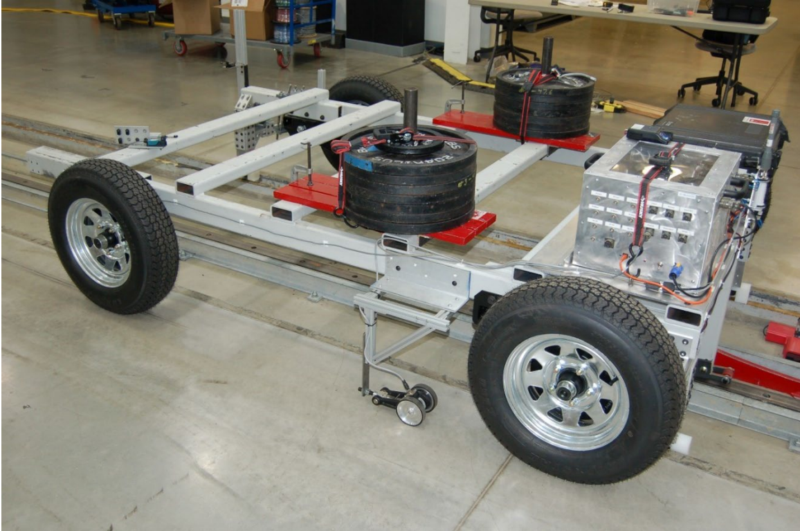
Figure 34: Sled Cart Used for ROV Debris Penetration Tests
