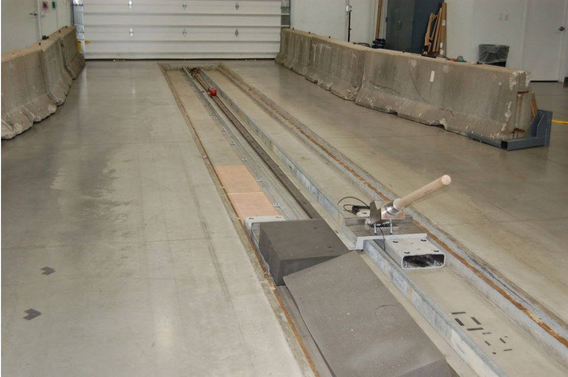
Figure 36: Stick and Stick Holder Mechanism – View Looking Down the Sled Track
