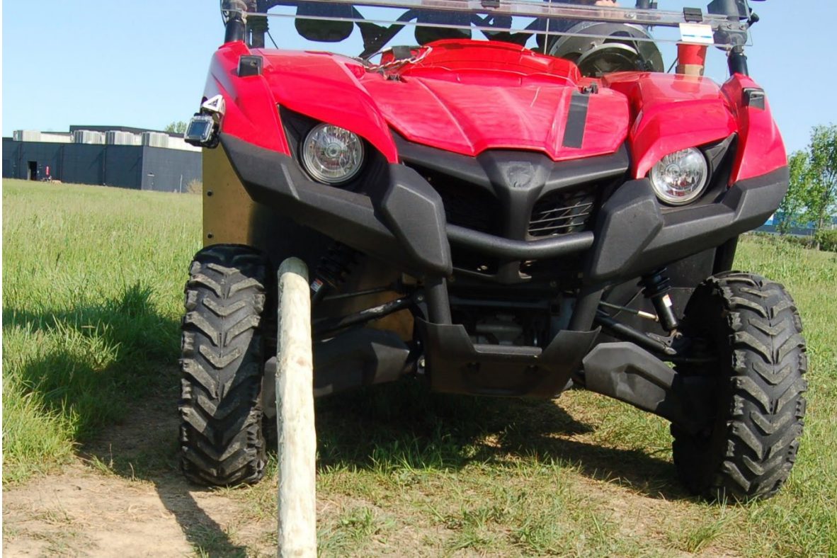
Figure 27: Vehicle D Run 2 Pre-Impact Stick Alignment – Front View
