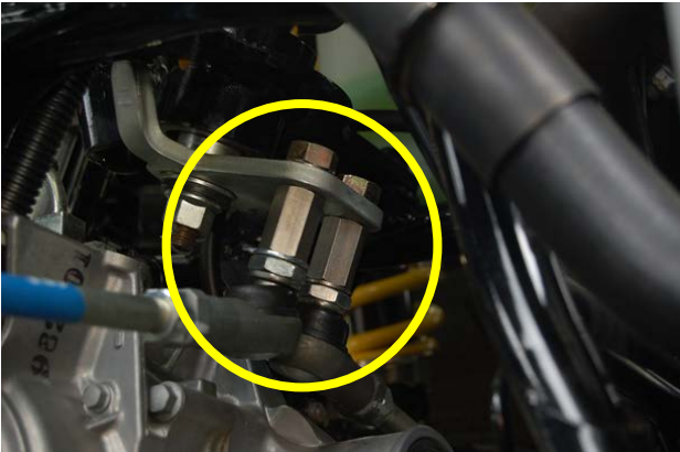
Modification 3 Steering Tie Rod Connections
