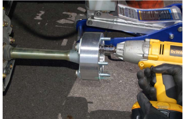
2" Wheel Spacer on Rear
