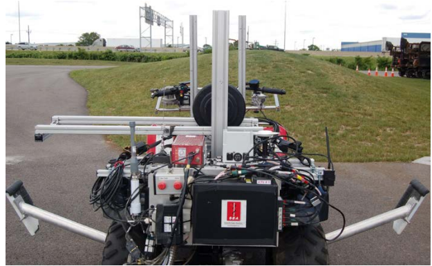
Lowered Rider-Lean Ballast Modification 2
