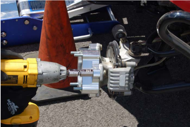
2" Wheel Spacer on Front
