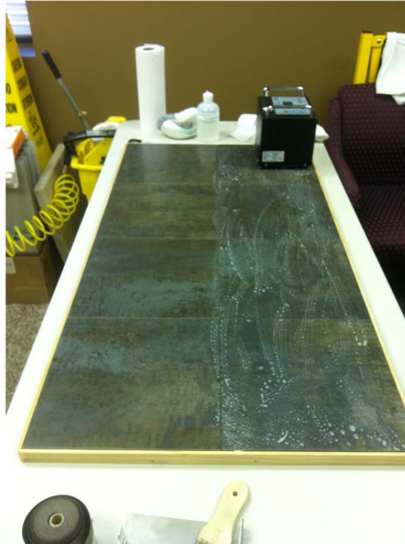
Figure 1 - Photo and configuration of the test rig used for DCOF testing.
