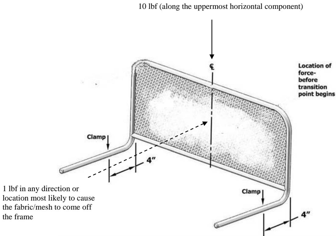
Figure 8: Determining misassembly/functional portable bed rail test setup
