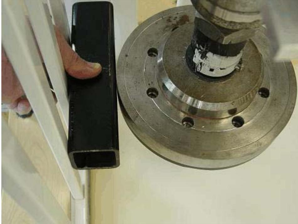
Figure D. Impact Mass and Spacer block (top view)Block
