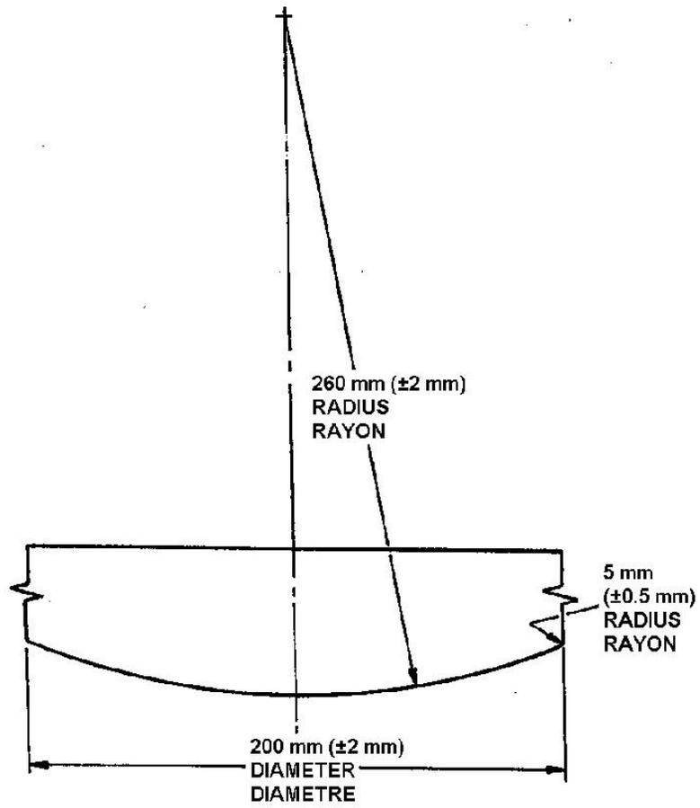
Figure A. Typical test frame Impactor Mass Shape
