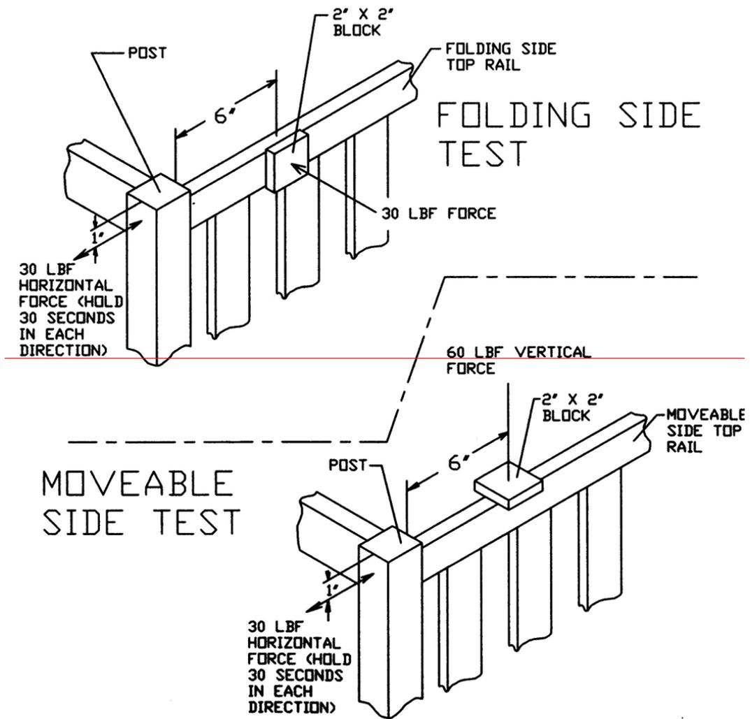
**Figure F. Side Latch Test**
