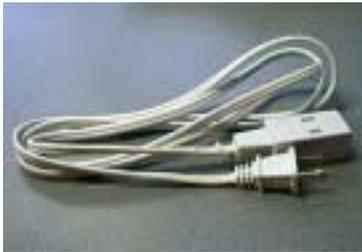
*Evaluate and test various extension cords to examine the failure mechanisms that lead to fires. Electrical overloads can increase fire risk when cords in use are undersized or the connections with or to the plug and receptacle are degraded from aging, oxidation or mechanical fatigue.*
