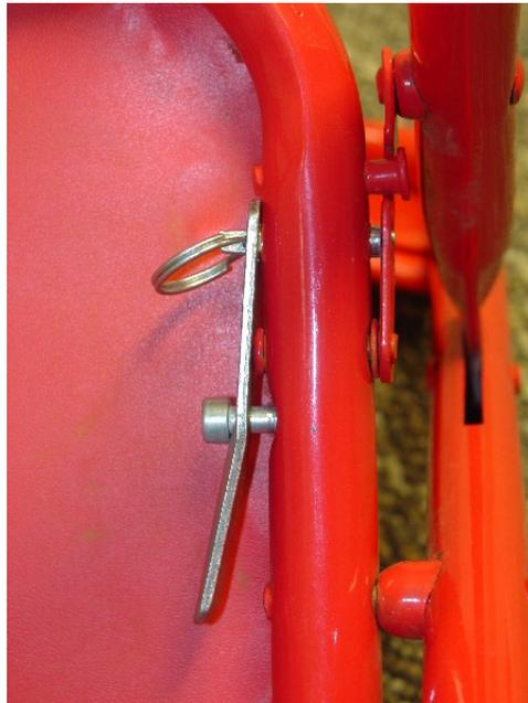
Figure 2. Spring-Loaded Locking Pin Mechanism
