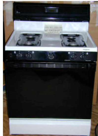
Figure 4. Gas Range used in Delayed-Ignition Tests
