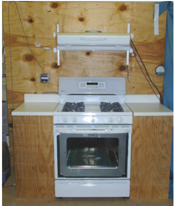
Figure 12. Gas Range and Range Hood used in Suction-Draft Tests
