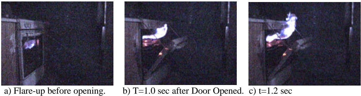
Figure 19. Opening Oven Door of Suction-Draft Range after Failed Combustion
