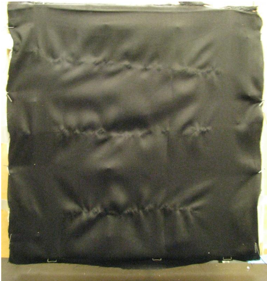
Photo 2 - Front view of the target, showing the cloth covering. Thermocouple junctions are in contact with the back side of the cloth.
