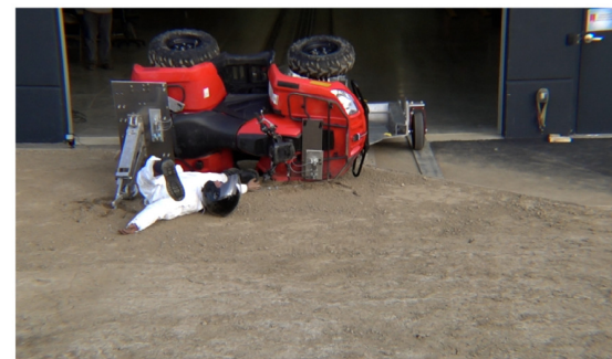
Drone Camera - End of Run - Roll Angle = 107.0°
