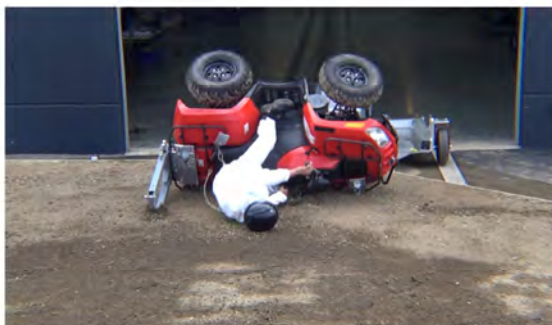
Drone Camera - ATD Head Strike - Time = 1.11 sec
