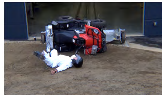
Drone Camera - End of Run - Roll Angle = 97.8°
