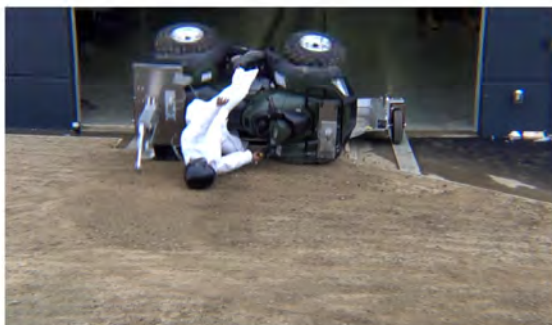
Drone Camera - ATD Head Strike - Time = 0.98 sec
