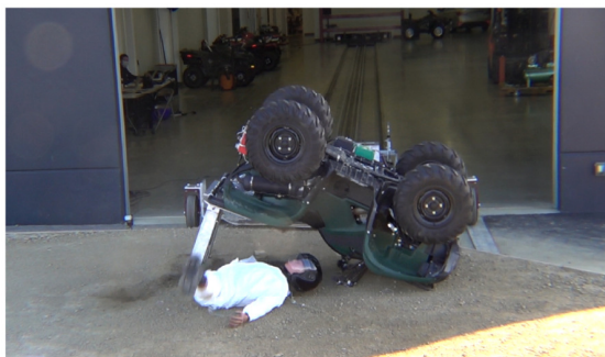
Drone Camera - Roll Angle = 180° - Time = 1.46 sec
