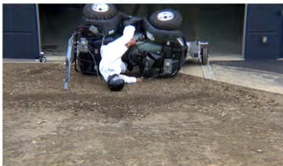
Drone Camera - ATD Head Strike - Time = 0.86 sec
