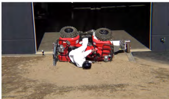
Drone Camera - ATD Head Strike - Time = 0.82 sec
