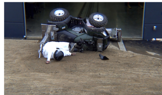
Drone Camera - End of Run - Roll Angle = 118.0°
