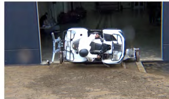
Drone Camera - Roll Angle = 90° - Time = 0.72 sec
