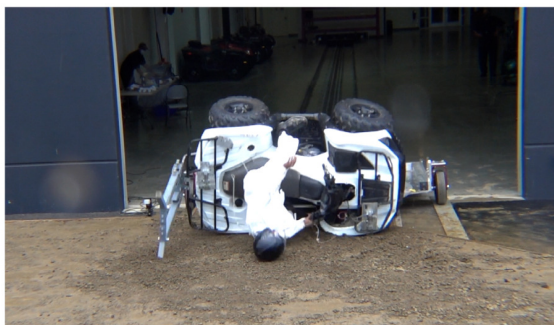
Drone Camera - ATD Head Strike - Time = 0.82 sec
