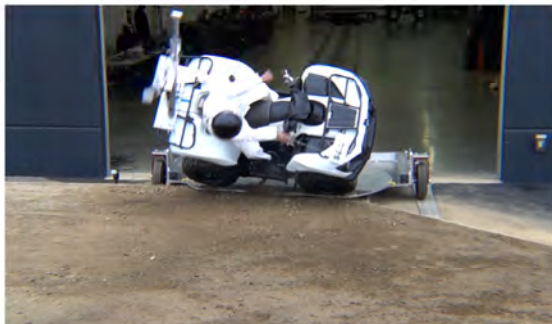
Drone Camera - Roll Angle = 30° - Time = 0.55 sec
