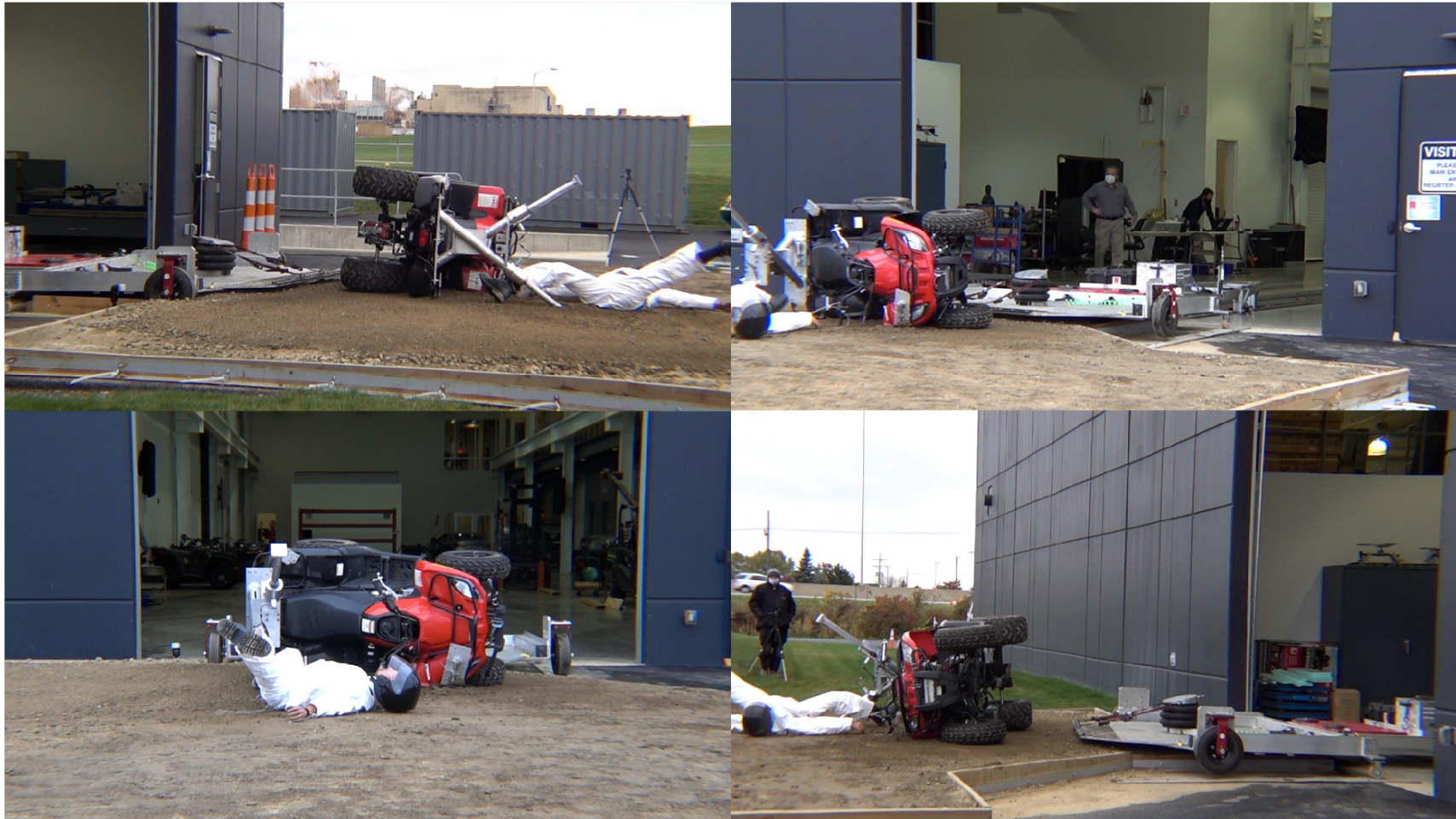
Vehicle F - Sled Moderate Energy Rollover – POC #3 – Extended Span OPD
