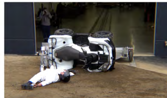
Drone Camera - End of Run - Roll Angle = 99.1°
