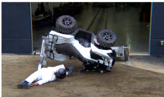
Drone Camera - Max Angle = 130.0° - Time = 1.55 sec
