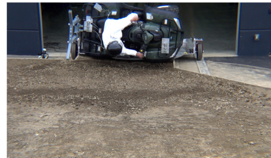
Drone Camera - Roll Angle = 90° - Time = 0.76 sec
