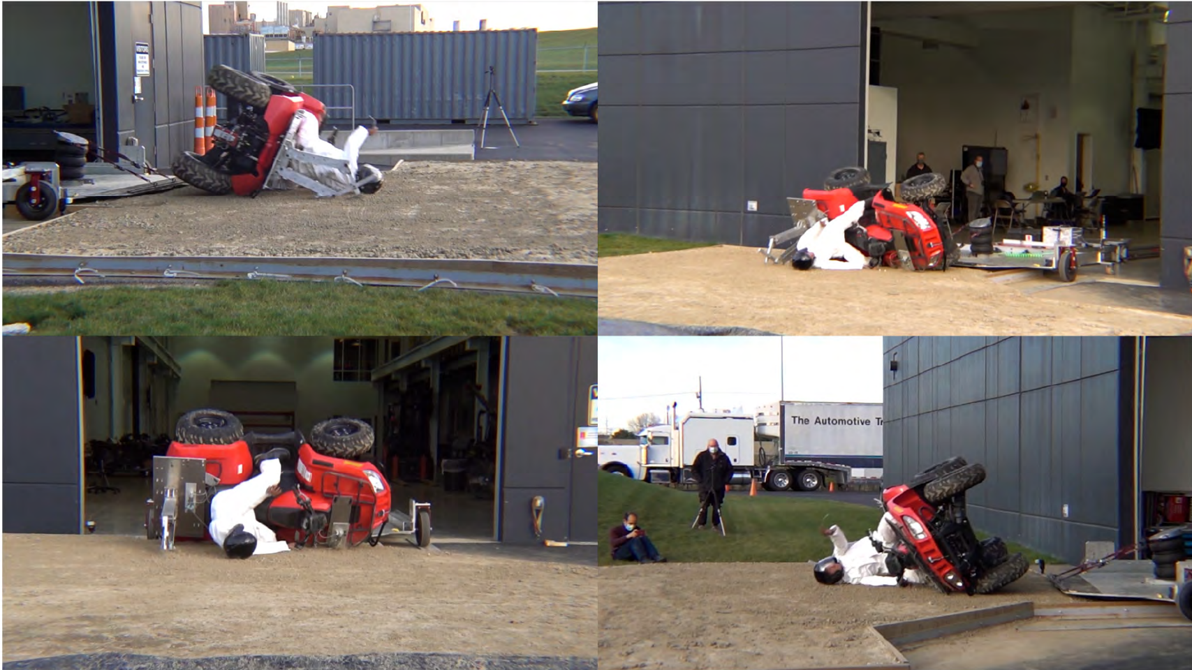
Vehicle E - Sled Moderate Energy Rollover – POC #5 – Extended Span OPD
