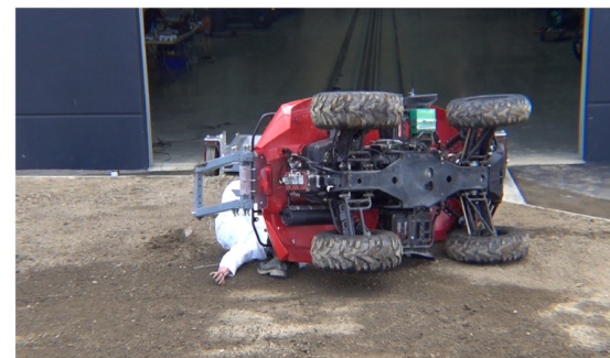
Drone Camera - Roll Angle = 270° - Time = 2.73 sec
