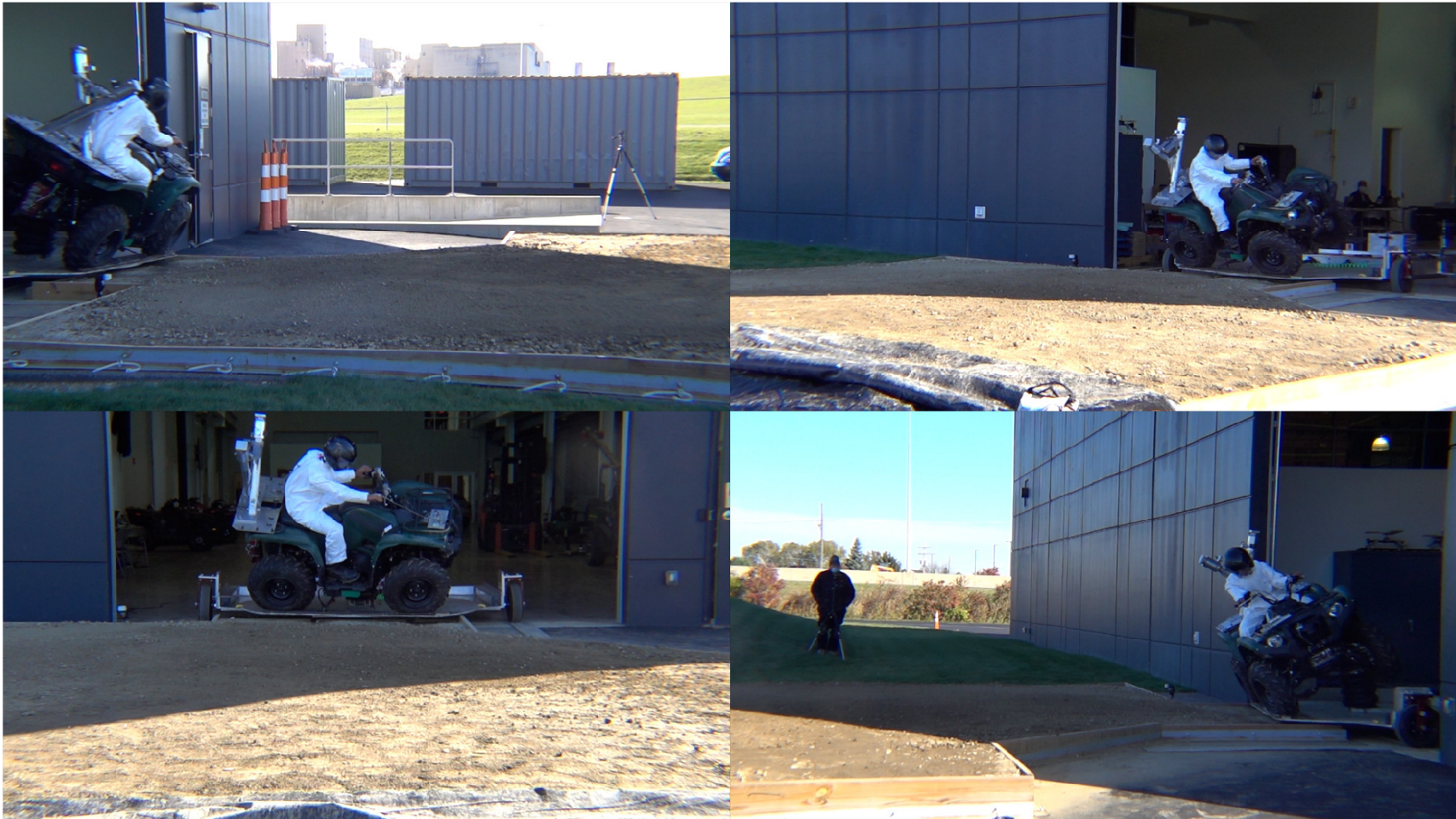
Vehicle C - Sled Moderate Energy Rollover – POC #3 Extra – Extended Span OPD
