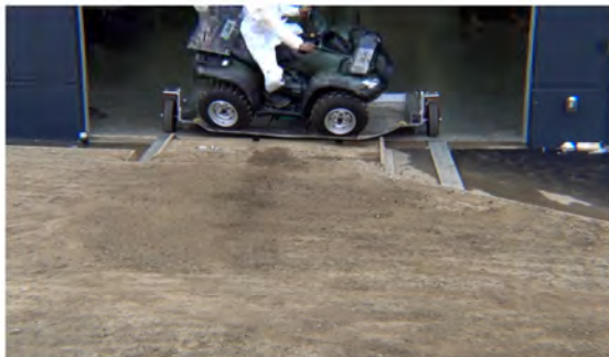
Drone Camera - Roll Angle = 30° - Time = 0.52 sec
