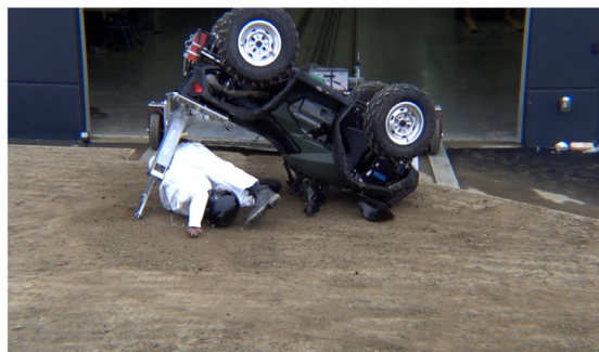
Drone Camera - Max Angle = 171.5° - Time = 2.08 sec
