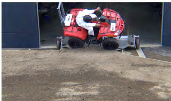
Drone Camera - Roll Angle = 45° - Time = 0.68 sec
