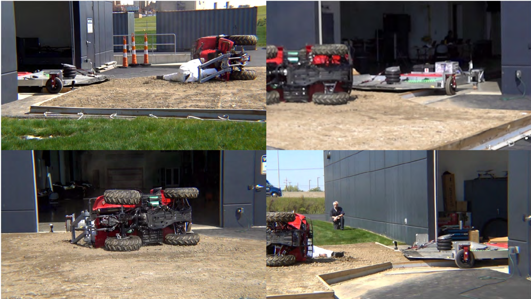
Vehicle A - Sled Moderate Energy Rollover – POC #2 – Energy Absorbing OPD
