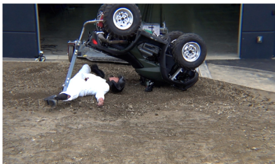
Drone Camera - Max Angle = 174.2° - Time = 1.62 sec
