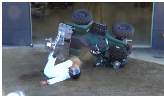
Drone Camera - Max Angle = 115.4° - Time = 1.51 sec
