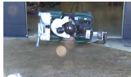
Drone Camera - Roll Angle = 90° - Time = 0.93 sec
