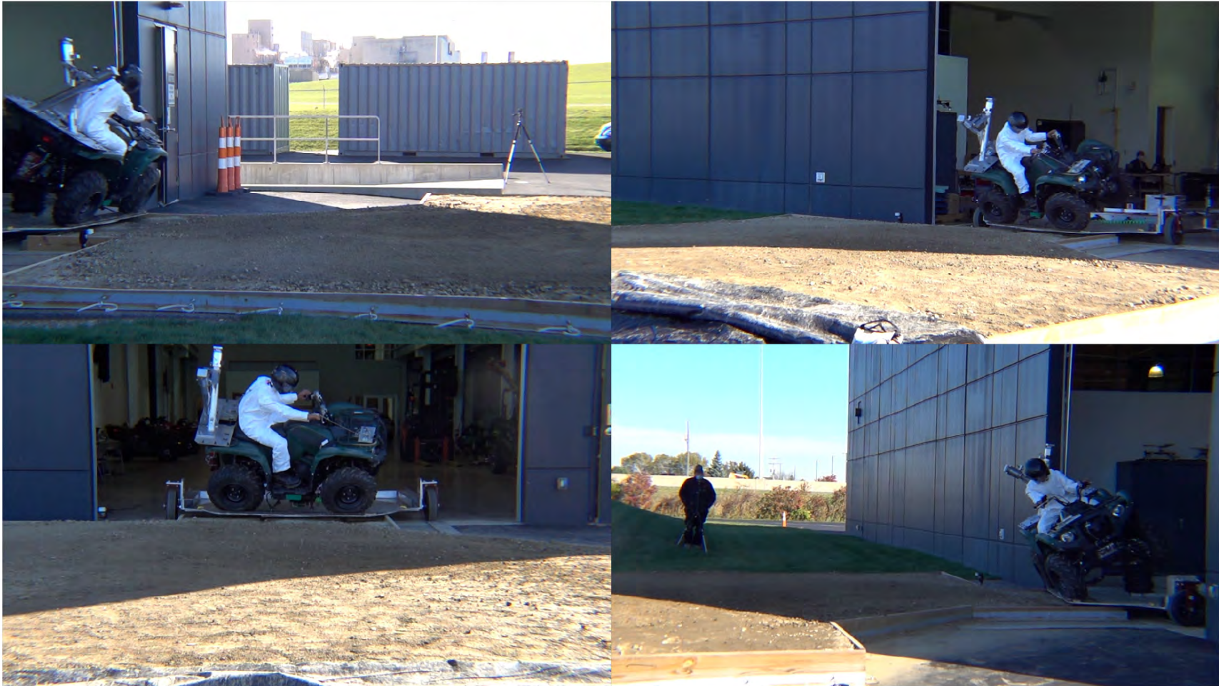
Vehicle C - Sled Moderate Energy Rollover – POC #3 Extra – Extended Span OPD
