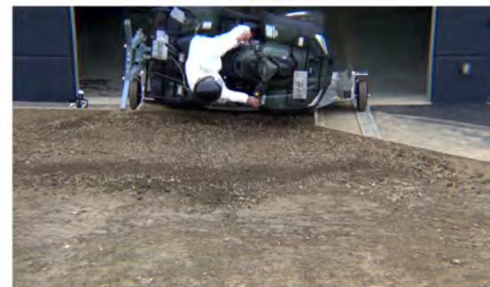
Drone Camera - Roll Angle = 90° - Time = 0.76 sec
