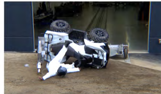
Drone Camera - Roll Angle = 90° - Time = 0.90 sec
