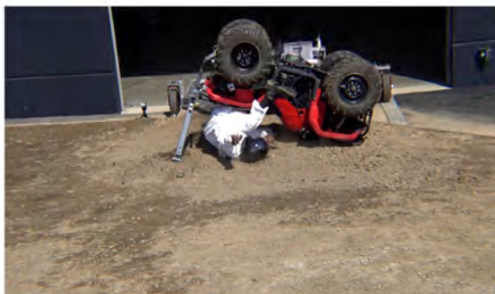
Drone Camera - Roll Angle = 180° - Time = 1.36 sec
