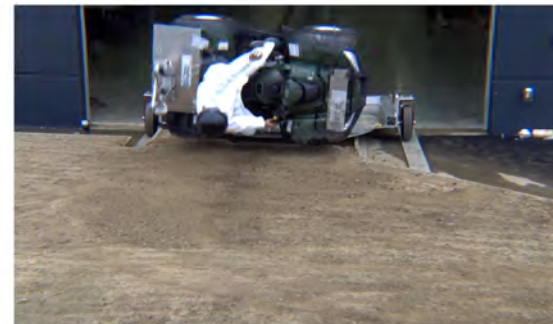
Drone Camera - Roll Angle = 90° - Time = 0.90 sec
