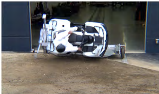
Drone Camera - Roll Angle = 45° - Time = 0.67 sec
