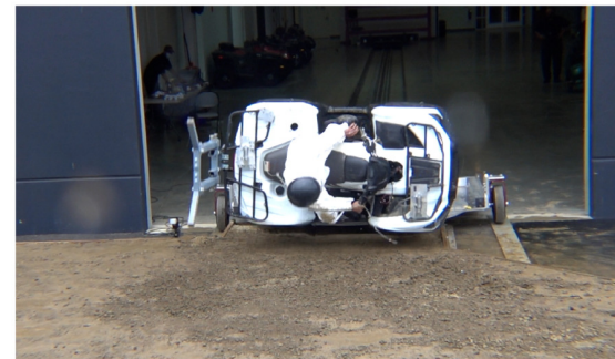
Drone Camera - Roll Angle = 90° - Time = 0.72 sec
