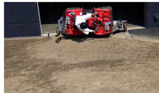
Drone Camera - Roll Angle = 90° - Time = 0.80 sec
