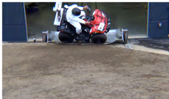
Drone Camera - Roll Angle = 45° - Time = 0.72 sec
