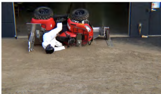
Drone Camera - ATD Head Strike - Time = 1.05 sec
