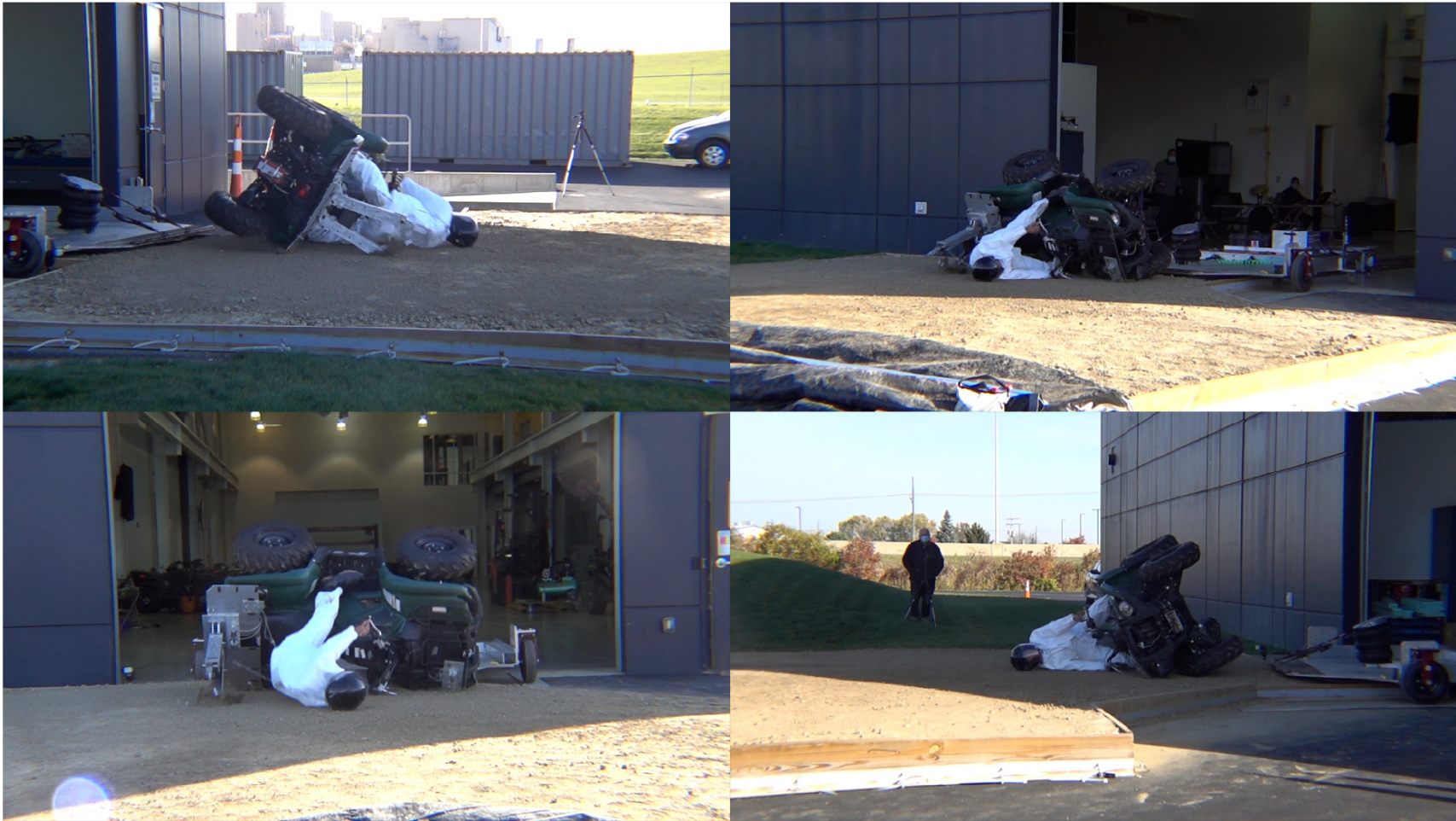
Vehicle C - Sled Moderate Energy Rollover – POC #4 – Energy Absorbing OPD
