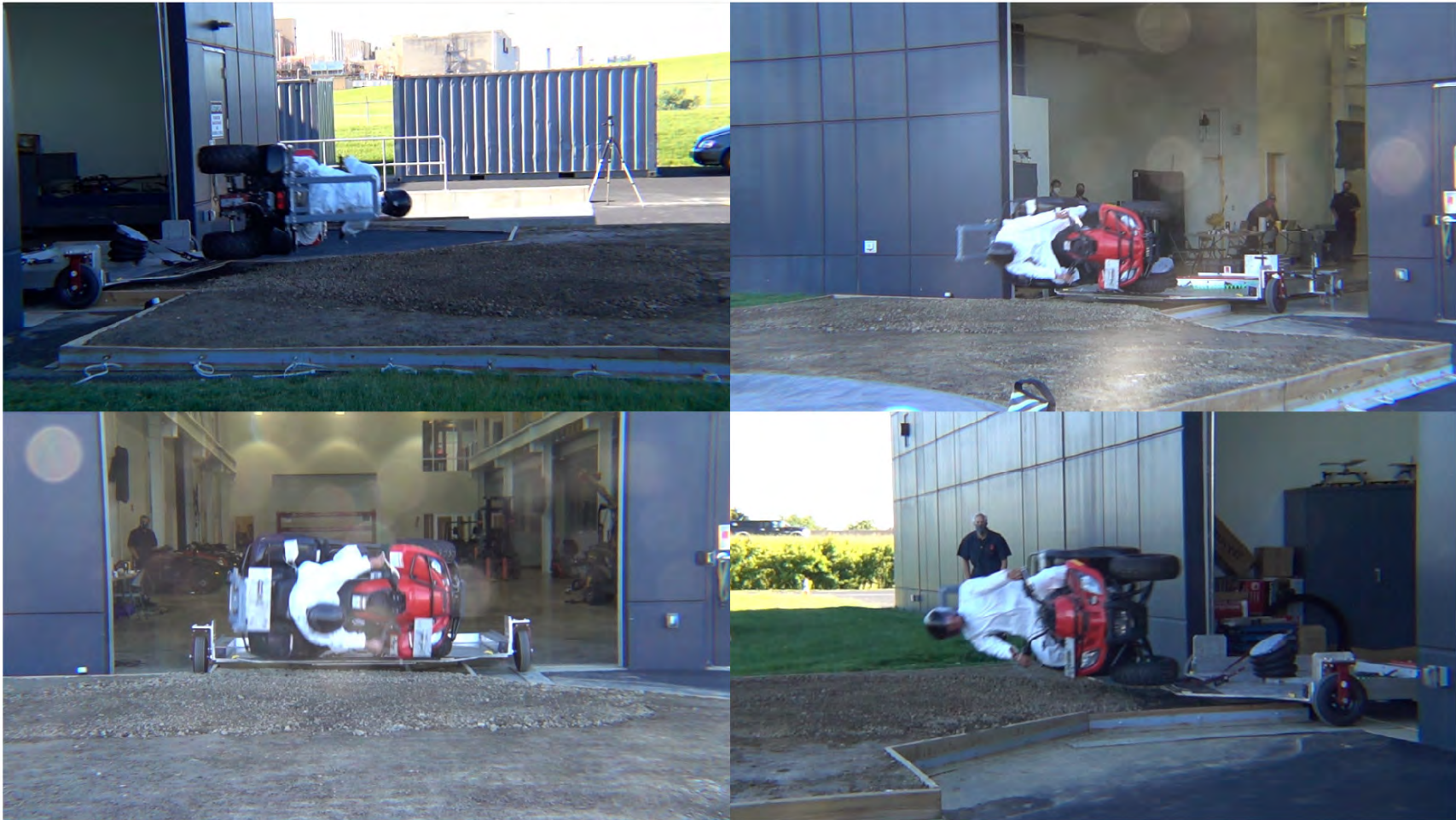
Vehicle F - Sled Moderate Energy Rollover – POC #2 – Energy Absorbing OPD
