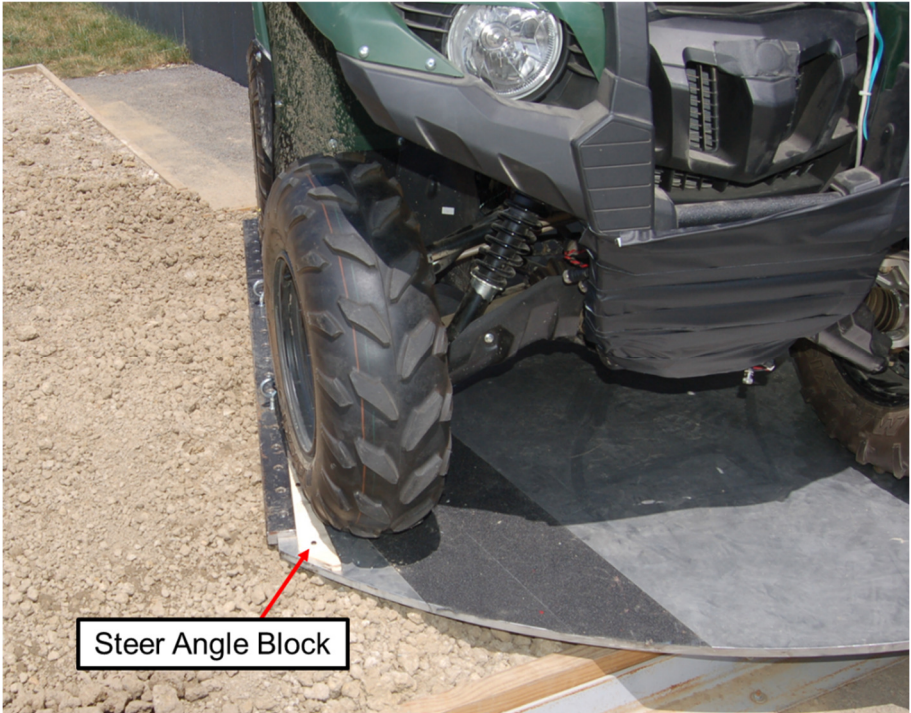
Figure B.5: Photo Showing Steer Angle Block
