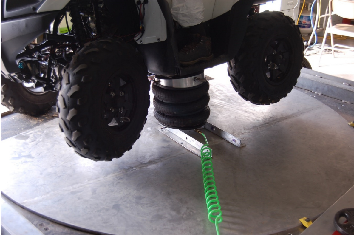
Figure B.6: Photo Showing Helper Spring used to Set ATV Initial Roll Angle
