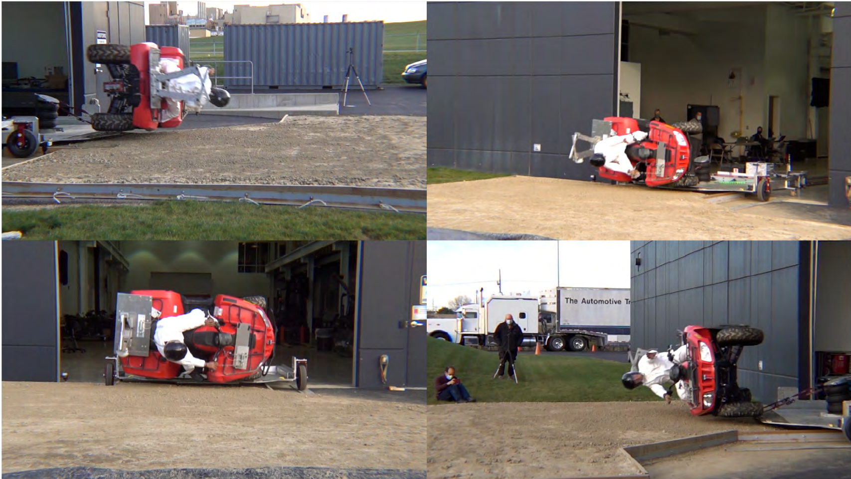
Vehicle E - Sled Moderate Energy Rollover – POC #5 – Extended Span OPD
