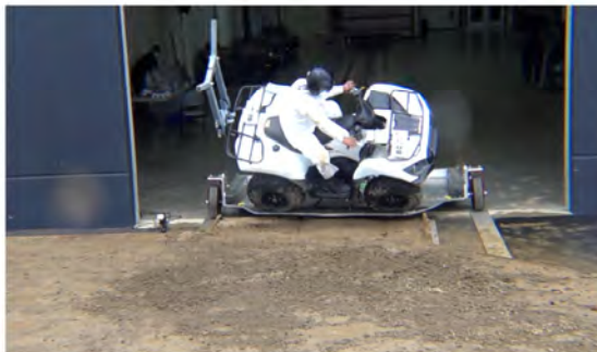
Drone Camera - Roll Angle = 45° - Time = 0.48 sec
