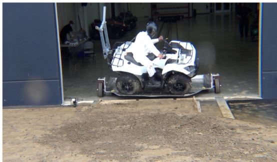
Drone Camera - Roll Angle = 30° - Time = 0.36 sec
