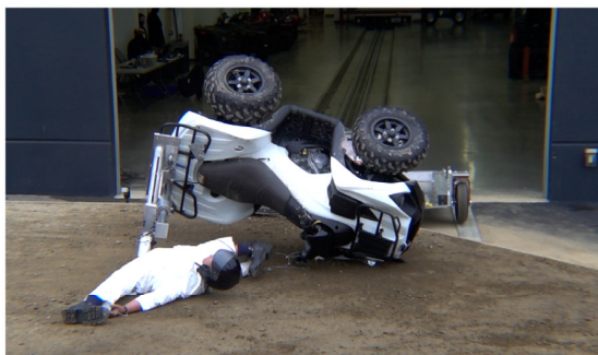
Drone Camera - Max Angle = 130.0° - Time = 1.55 sec
