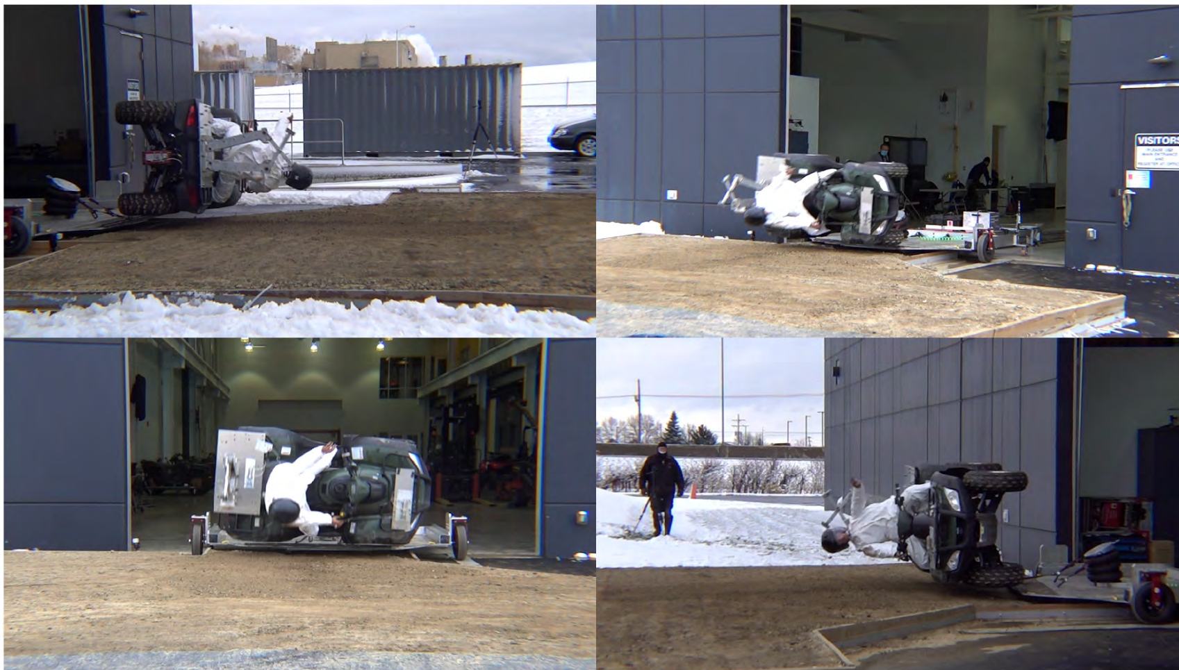
Vehicle J - Sled Moderate Energy Rollover – POC #5 – Extended Span OPD
