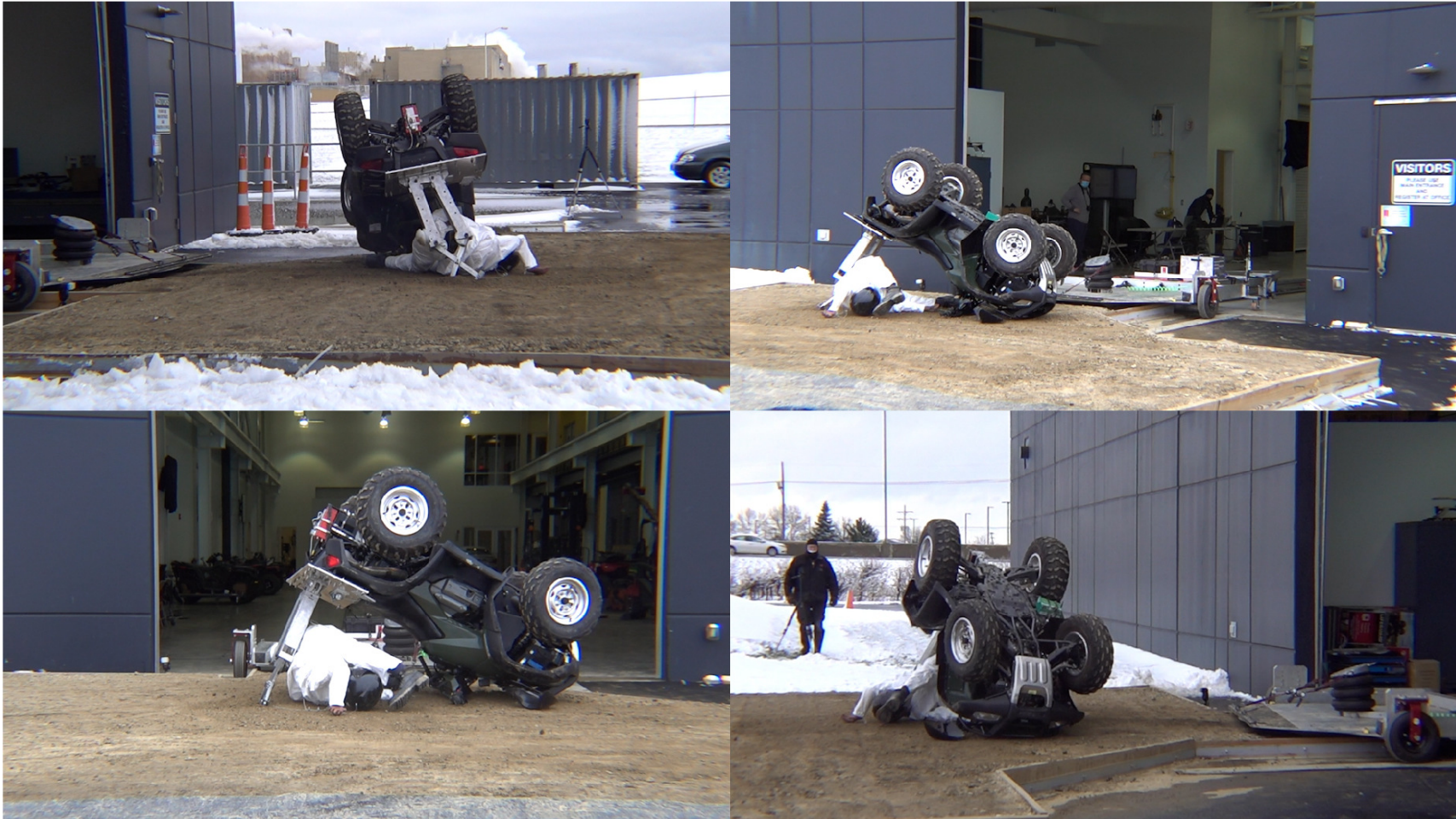
Vehicle J - Sled Moderate Energy Rollover – POC #5 – Extended Span OPD
