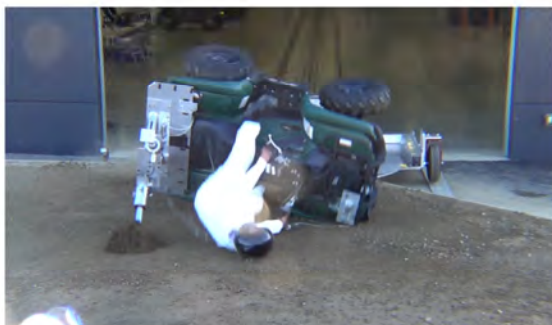
Drone Camera - ATD Head Strike - Time = 1.11 sec
