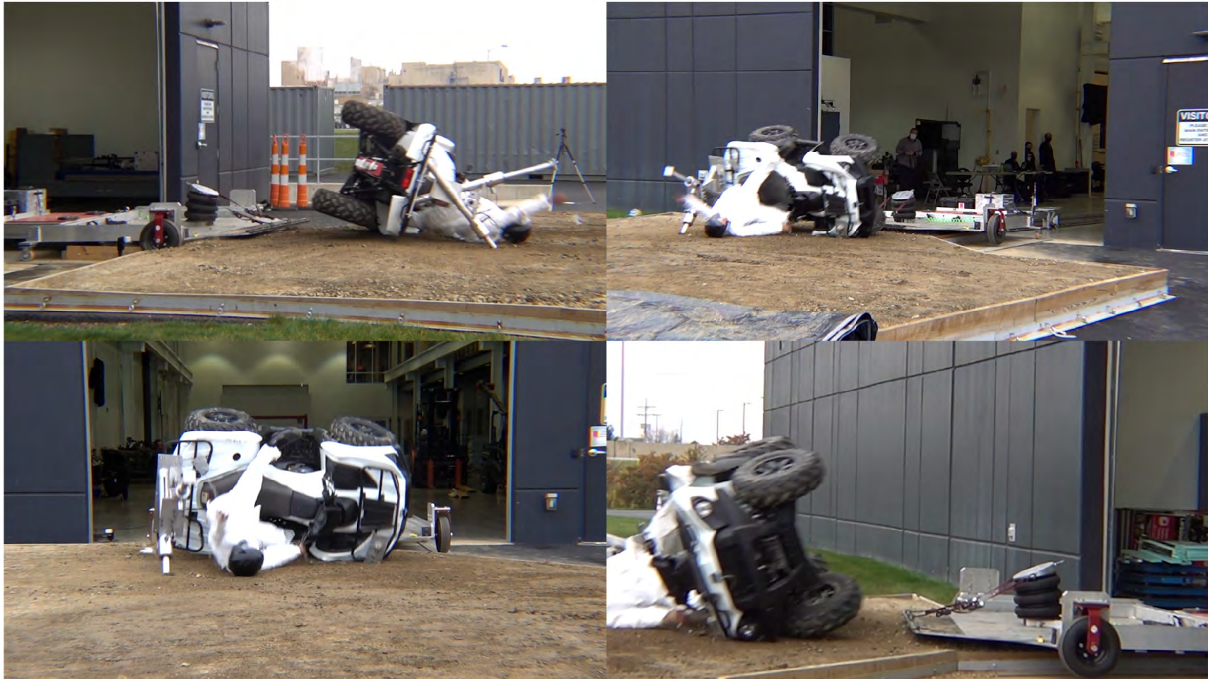
Vehicle G - Sled Moderate Energy Rollover – POC #3 – Extended Span OPD
