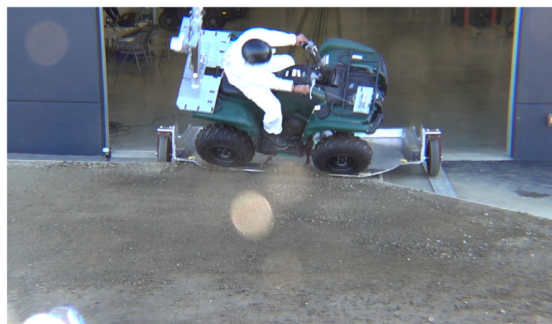
Drone Camera - Roll Angle = 45° - Time = 0.69 sec
