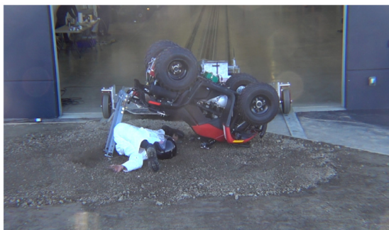
Drone Camera - Roll Angle = 180° - Time = 1.47 sec
