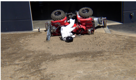
Drone Camera - ATD Head Strike - Time = 0.94 sec
