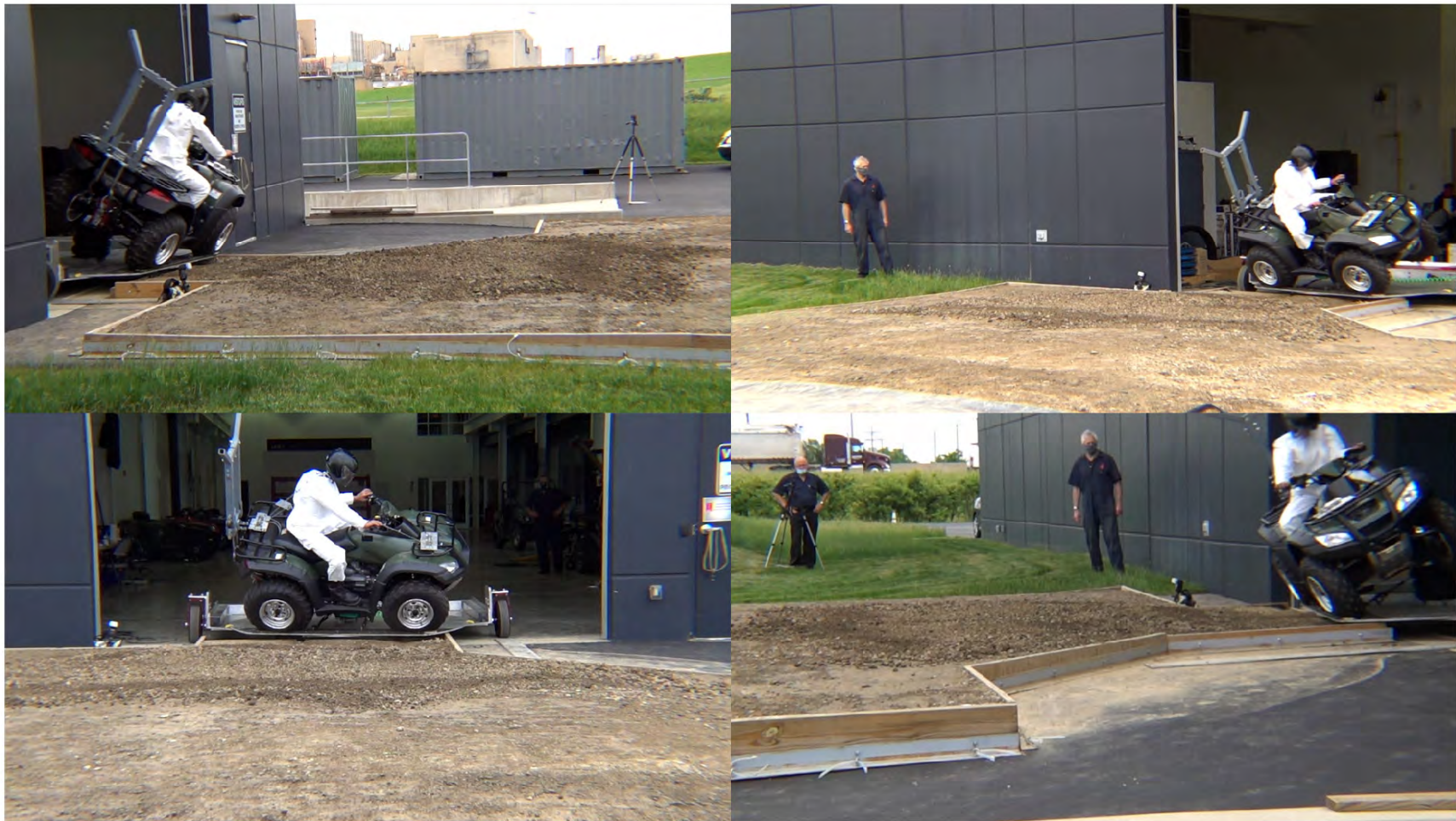
Vehicle J - Sled Moderate Energy Rollover – POC #1 – Extended Span OPD
