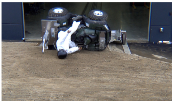
Drone Camera - ATD Head Strike - Time = 0.98 sec
