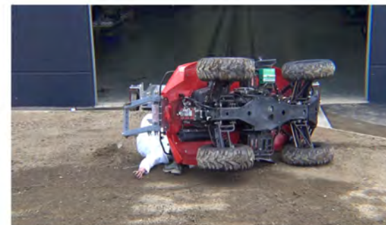
Drone Camera - Roll Angle = 270° - Time = 2.73 sec
