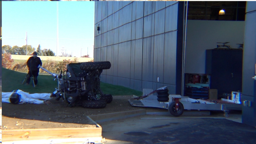
Vehicle C - Sled Moderate Energy Rollover – POC #3 – Extended Span OPD
