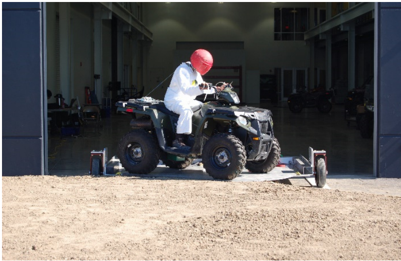
Figure B.1: Views of ATV Rollover Simulator Along the Direction of Sled Translation
