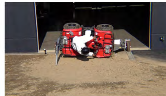
Drone Camera - Roll Angle = 90° - Time = 0.74 sec
