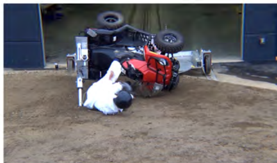
Drone Camera - Max Angle = 113.0° - Time = 1.26 sec
