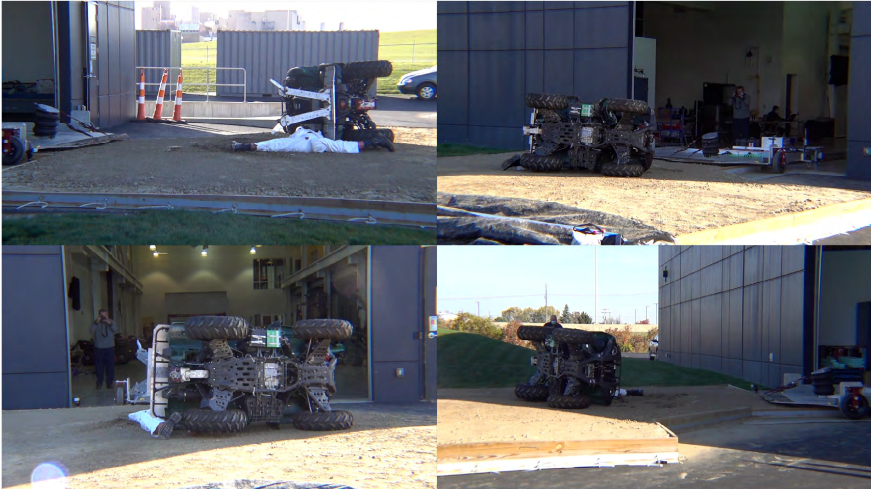
Vehicle C - Sled Moderate Energy Rollover – POC #4 – Energy Absorbing OPD
