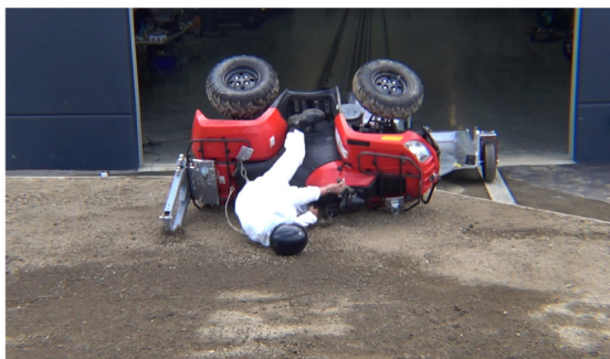
Drone Camera - ATD Head Strike - Time = 1.11 sec
