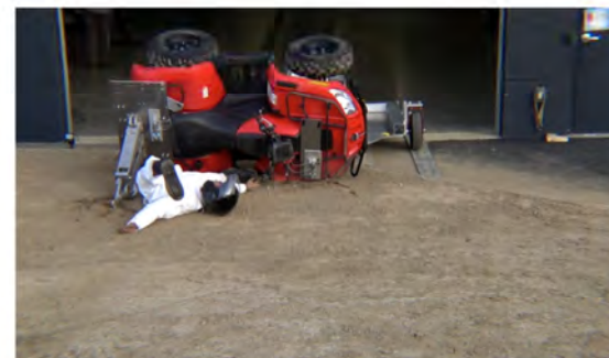
Drone Camera - End of Run - Roll Angle = 107.0°
