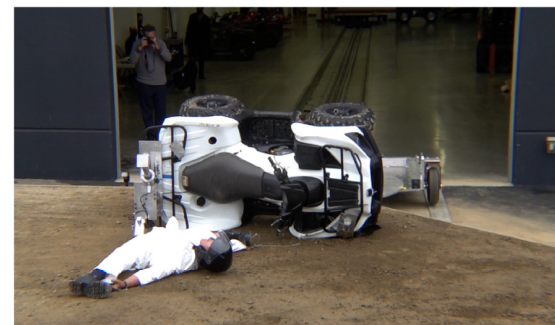
Drone Camera - End of Run - Roll Angle = 99.1°
