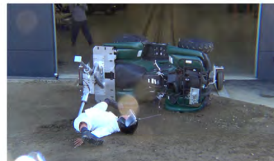
Drone Camera - End of Run - Roll Angle = 96.7°
