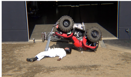
Drone Camera - Max Angle = 167.6° - Time = 1.75 sec
