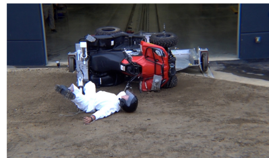
Drone Camera - End of Run - Roll Angle = 97.8°
