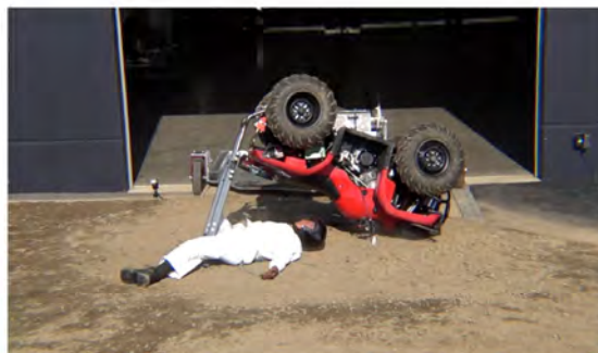
Drone Camera - Max Angle = 167.6° - Time = 1.75 sec
