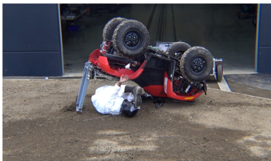
Drone Camera - Roll Angle = 180° - Time = 1.52 sec
