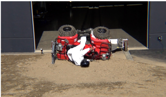
Drone Camera - ATD Head Strike - Time = 0.82 sec
