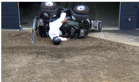
Drone Camera - ATD Head Strike - Time = 0.86 sec
