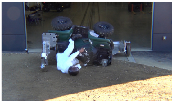
Drone Camera - ATD Head Strike - Time = 1.10 sec
