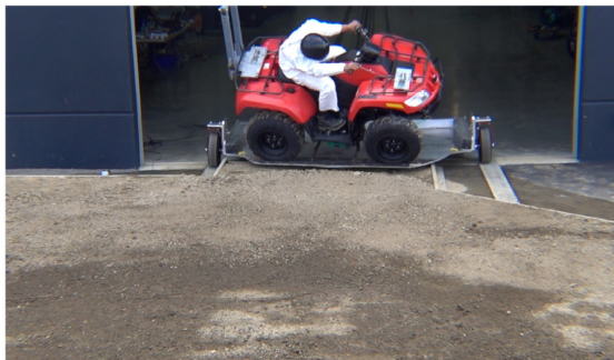
Drone Camera - Roll Angle = 30° - Time = 0.53 sec
