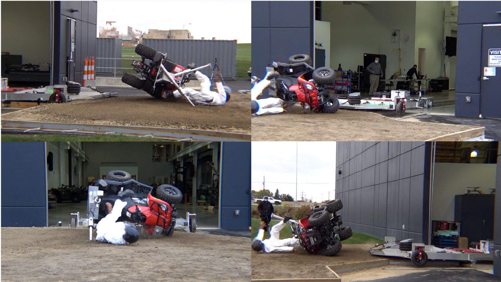
Vehicle F - Sled Moderate Energy Rollover – POC #3 – Extended Span OPD
