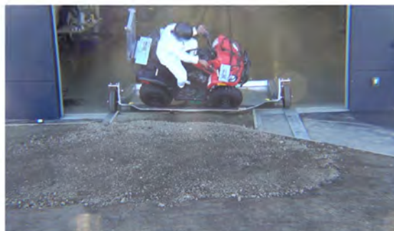
Drone Camera - Roll Angle = 45° - Time = 0.51 sec
