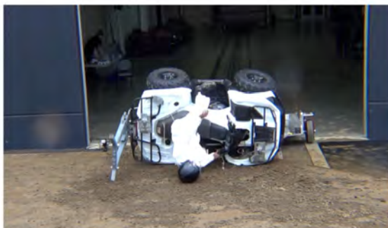
Drone Camera - ATD Head Strike - Time = 0.82 sec
