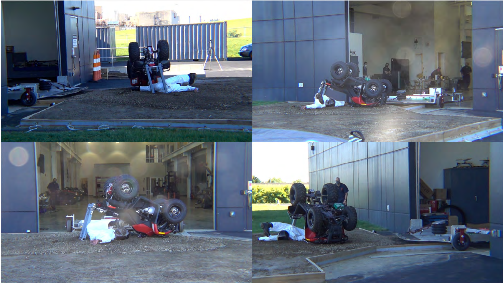
Vehicle F - Sled Moderate Energy Rollover – POC #2 – Energy Absorbing OPD
