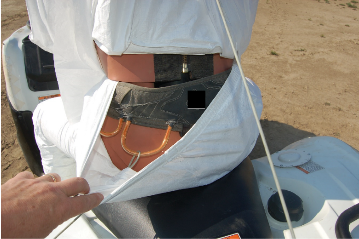
Figure D.5: Harness used for Attaching the Hip Cable to the ATD
