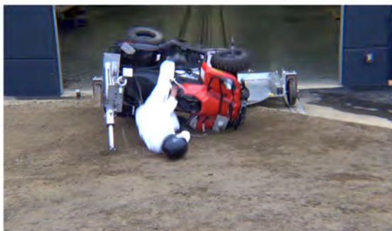
Drone Camera - ATD Head Strike - Time = 1.12 sec
