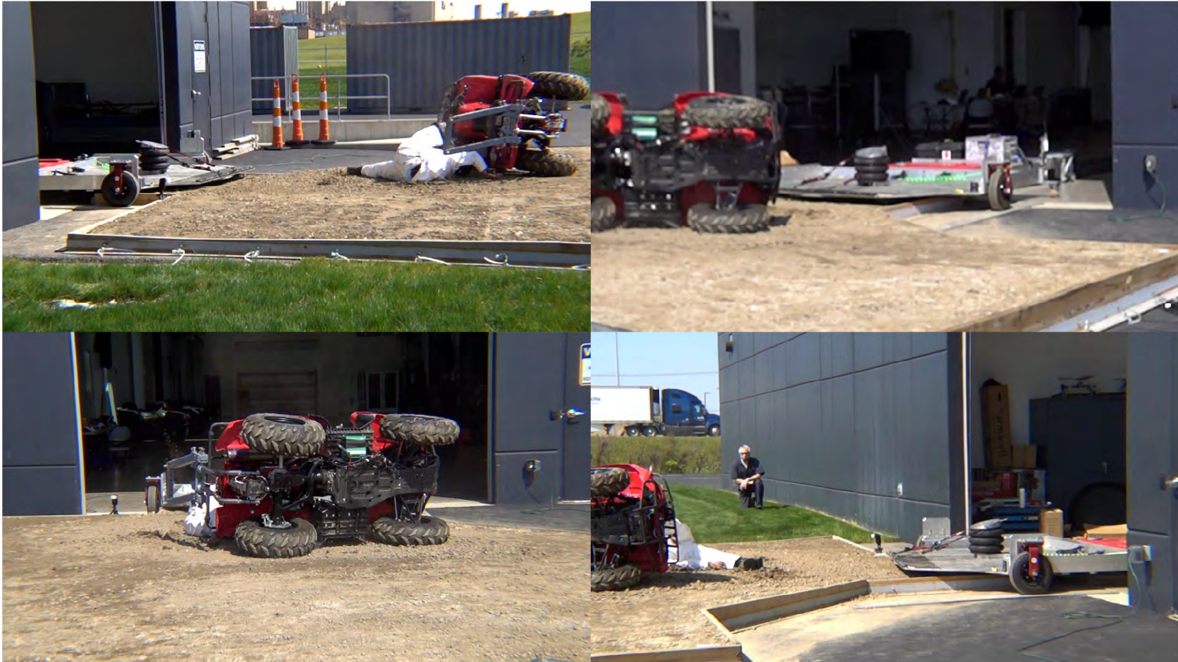
Vehicle A - Sled Moderate Energy Rollover – POC #2 – Energy Absorbing OPD
