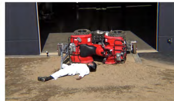
Drone Camera - End of Run - Roll Angle = 98.7°
