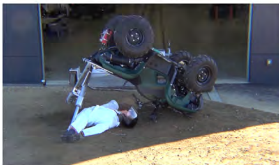
Drone Camera - Roll Angle = 180° - Time = 1.60 sec
