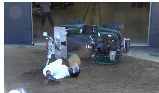
Drone Camera - End of Run - Roll Angle = 96.7°
