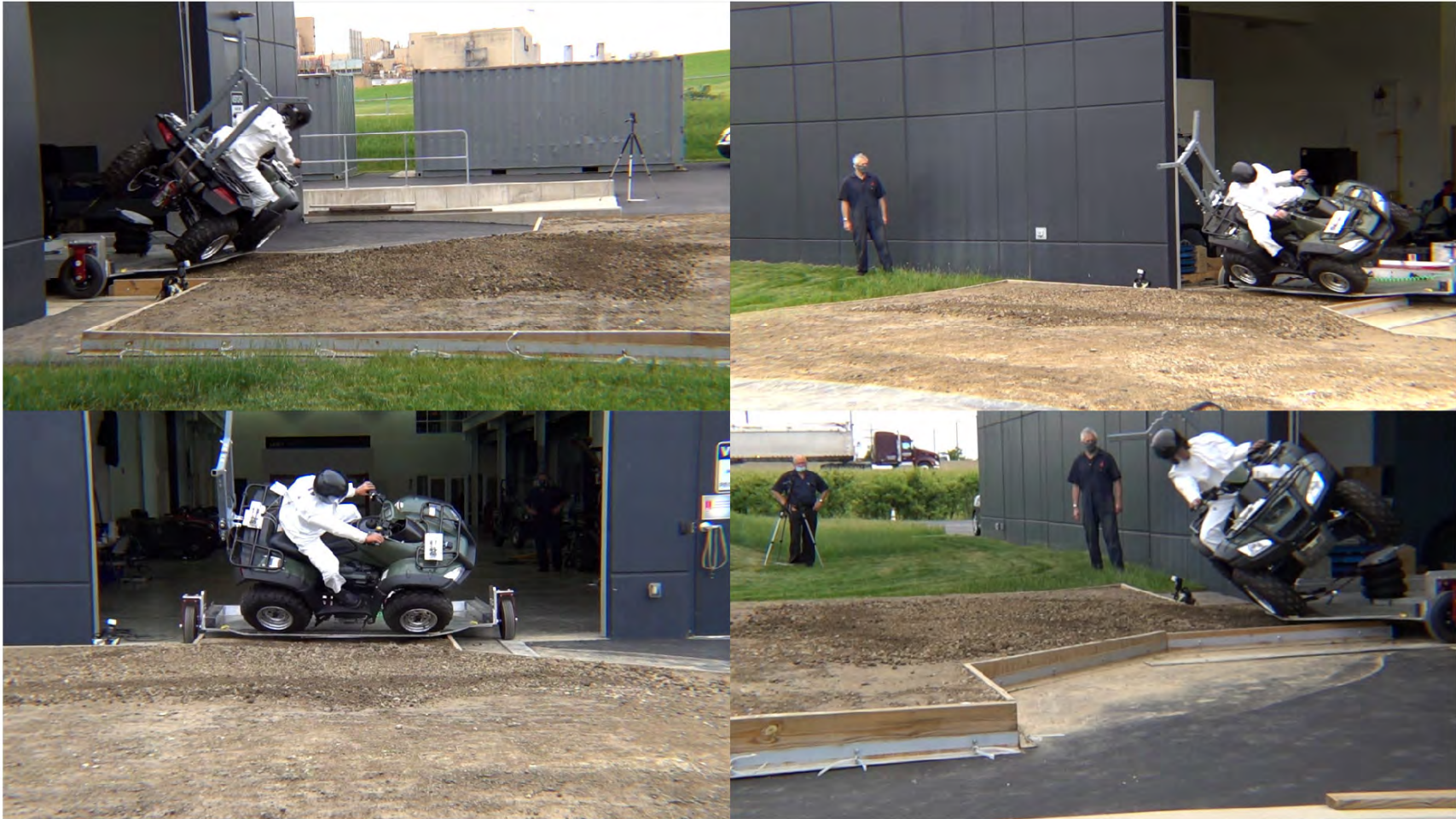
Vehicle J - Sled Moderate Energy Rollover – POC #1 – Extended Span OPD
