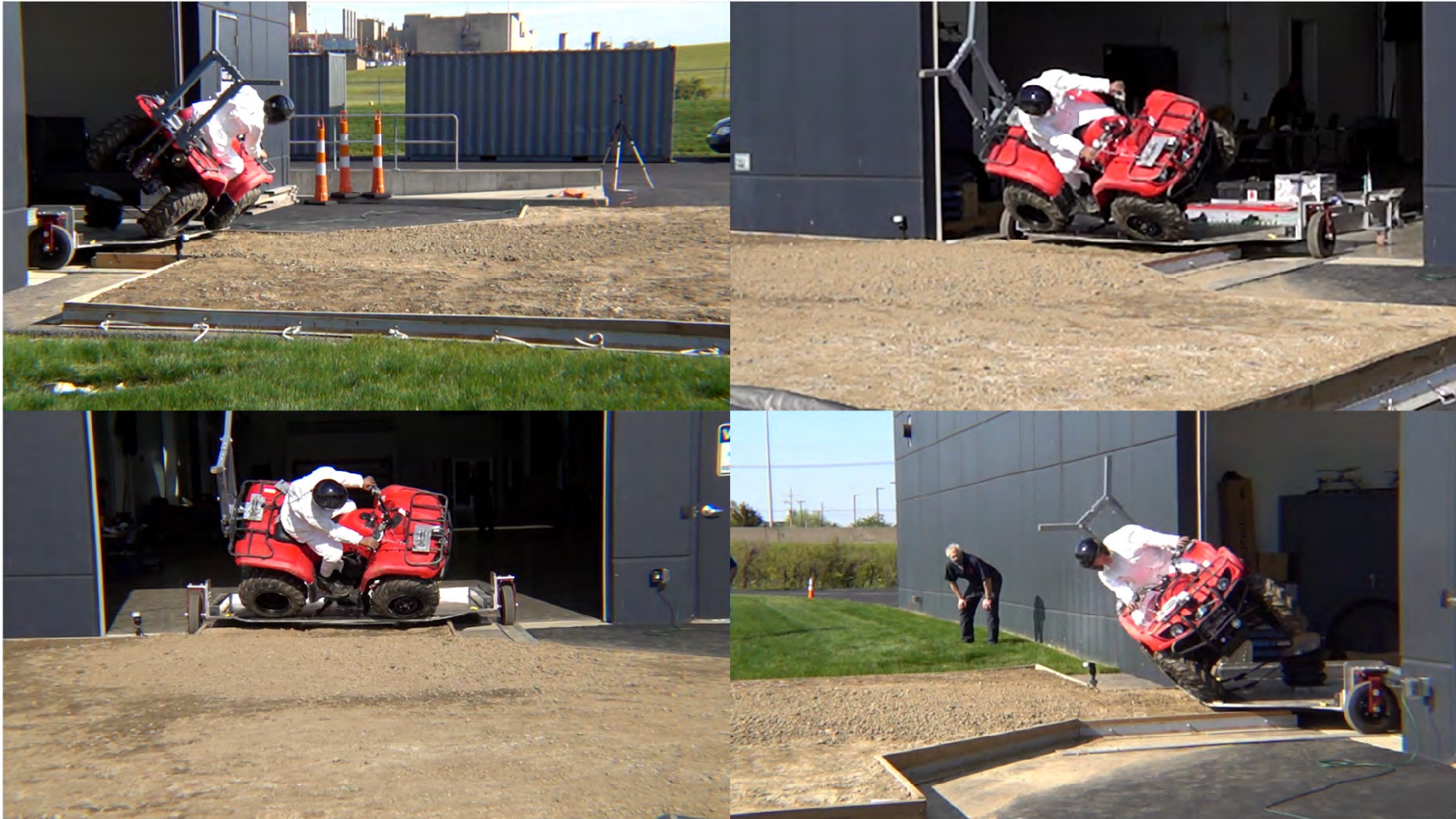
Vehicle A - Sled Moderate Energy Rollover – POC #1 – Extended Span OPD
