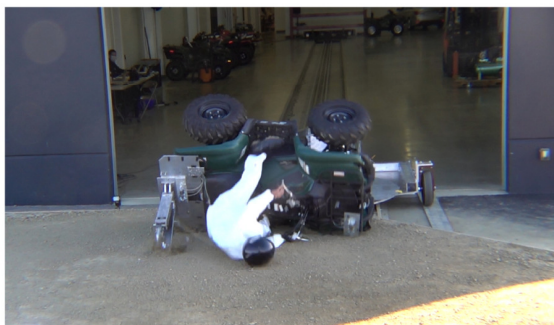
Drone Camera - ATD Head Strike - Time = 1.02 sec
