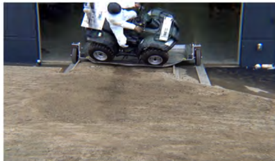
Drone Camera - Roll Angle = 45° - Time = 0.65 sec
