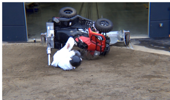
Drone Camera - Max Angle = 113.0° - Time = 1.26 sec
