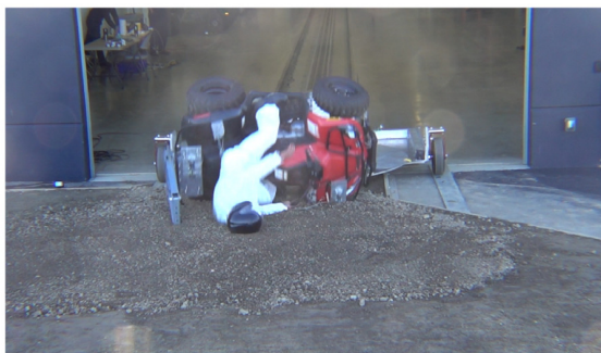
Drone Camera - ATD Head Strike - Time = 0.85 sec
