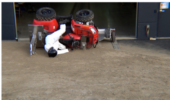
Drone Camera - ATD Head Strike - Time = 1.05 sec
