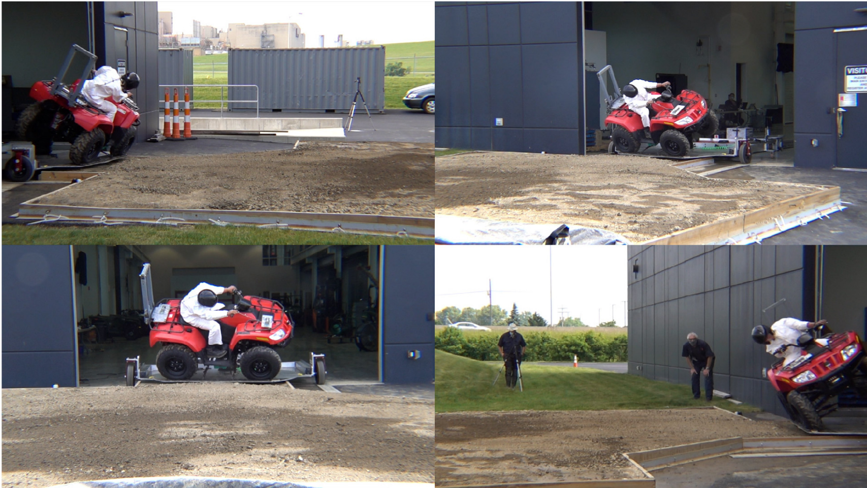
Vehicle E - Sled Moderate Energy Rollover – POC #2 – Energy Absorbing OPD
