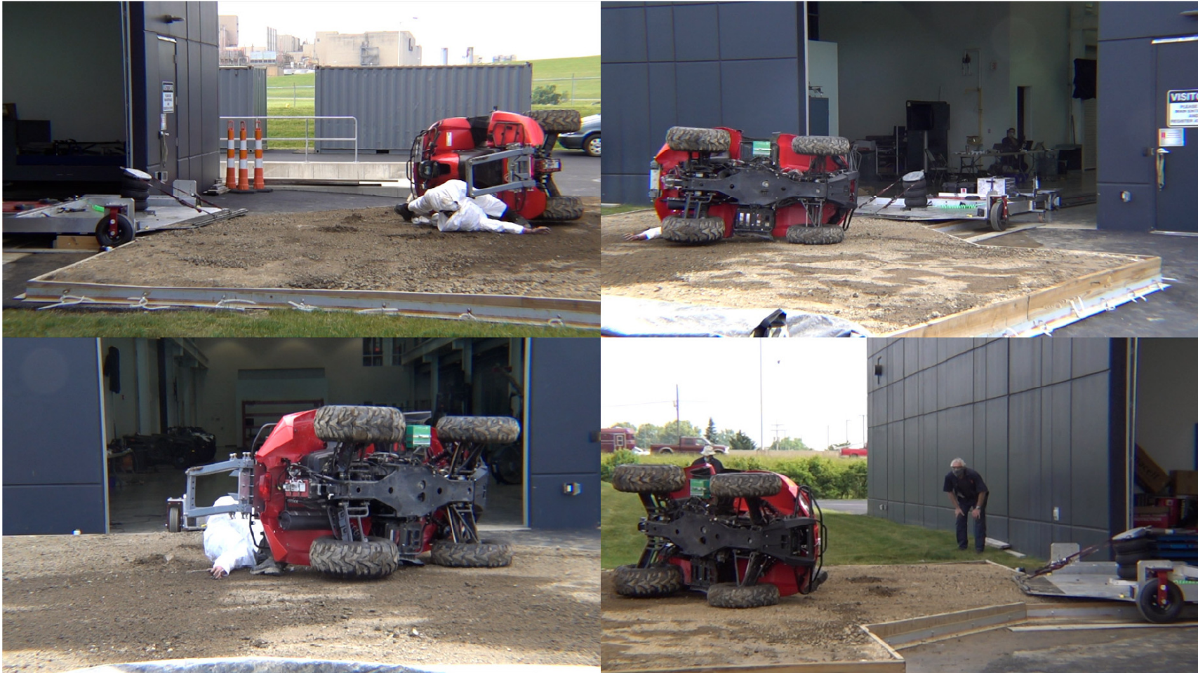
Vehicle E - Sled Moderate Energy Rollover – POC #2 – Energy Absorbing OPD
