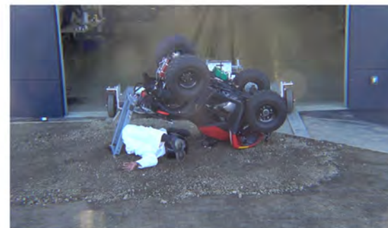
Drone Camera - Max Angle = 195.3° - Time = 1.88 sec
