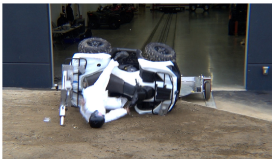
Drone Camera - ATD Head Strike - Time = 0.82 sec
