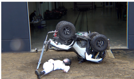
Drone Camera - Roll Angle = 180° - Time = 1.45 sec
