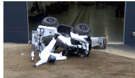
Drone Camera - Roll Angle = 90° - Time = 0.90 sec
