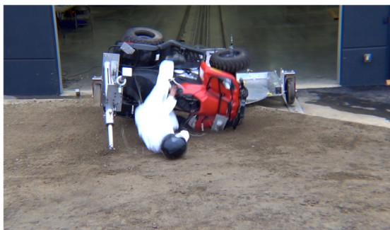
Drone Camera - ATD Head Strike - Time = 1.12 sec
