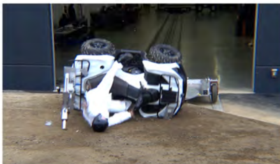
Drone Camera - ATD Head Strike - Time = 0.82 sec
