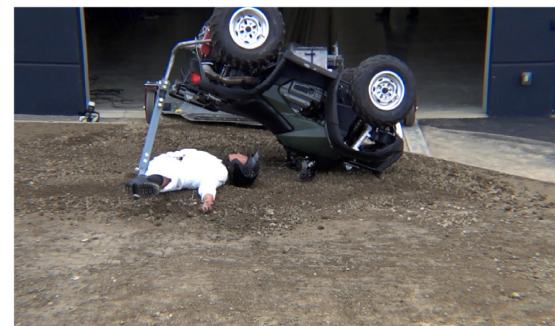
Drone Camera - End of Run - Roll Angle = 163.6°
