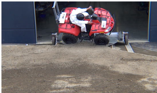
Drone Camera - Roll Angle = 45° - Time = 0.68 sec
