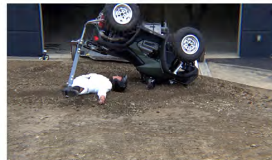
Drone Camera - End of Run - Roll Angle = 163.6°
