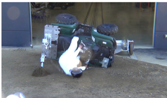
Drone Camera - ATD Head Strike - Time = 1.11 sec
