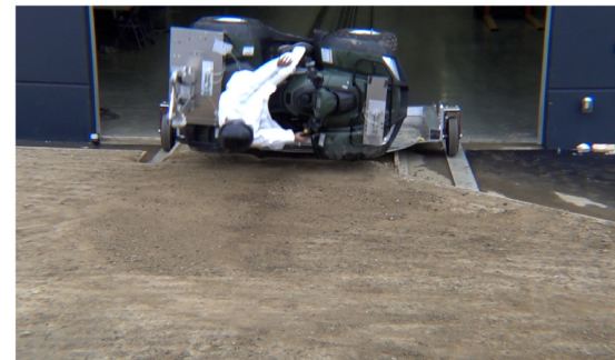
Drone Camera - Roll Angle = 90° - Time = 0.90 sec
