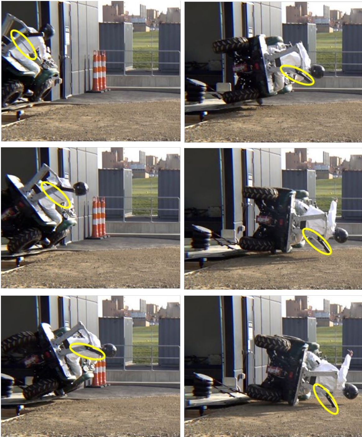
Figure 5: Free Swinging Aluminum Bar (Pointer) Attached to POC #4 to Demonstrate Acceleration Line of Action
