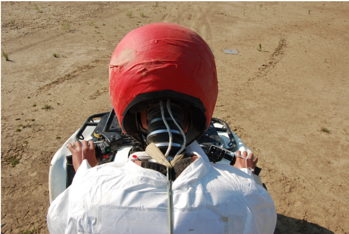
Figure D.6: Velcro Strap used for Attaching the Neck Cable to the ATD
