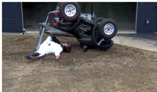
Drone Camera - Max Angle = 174.2° - Time = 1.62 sec
