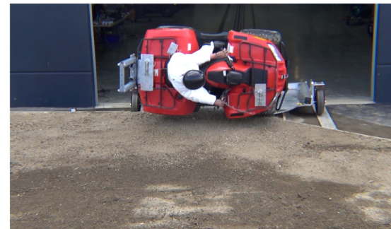
Drone Camera - Roll Angle = 90° - Time = 0.93 sec
