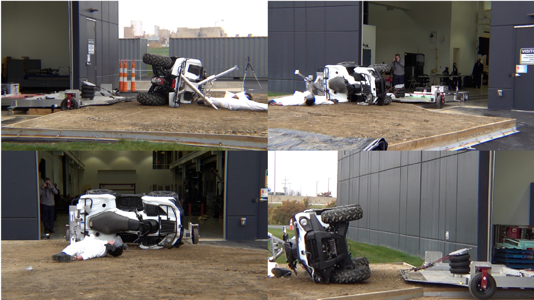
Vehicle G - Sled Moderate Energy Rollover – POC #3 – Extended Span OPD
