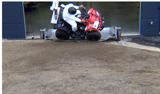
Drone Camera - Roll Angle = 45° - Time = 0.72 sec
