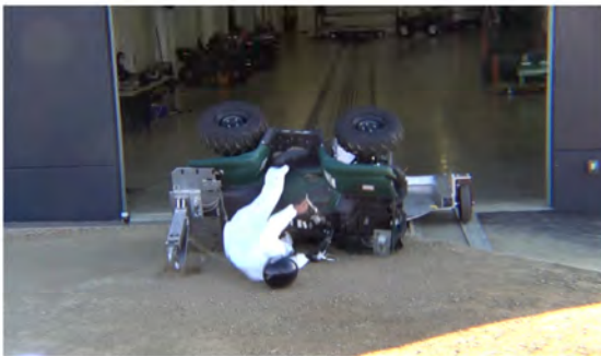
Drone Camera - ATD Head Strike - Time = 1.02 sec
