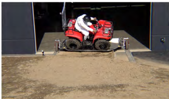
Drone Camera - Roll Angle = 30° - Time = 0.41 sec
