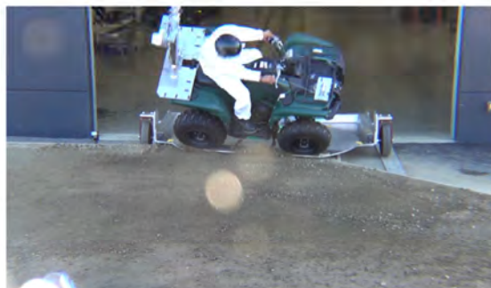
Drone Camera - Roll Angle = 45° - Time = 0.69 sec
