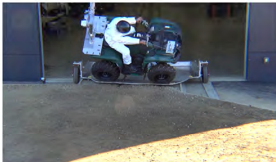
Drone Camera - Roll Angle = 45° - Time = 0.68 sec
