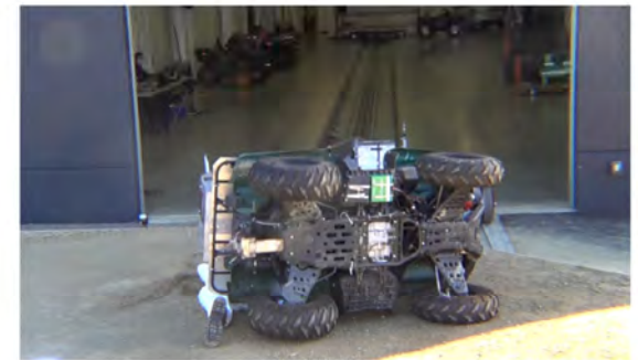
Drone Camera - Roll Angle = 270° - Time = 2.19 sec
