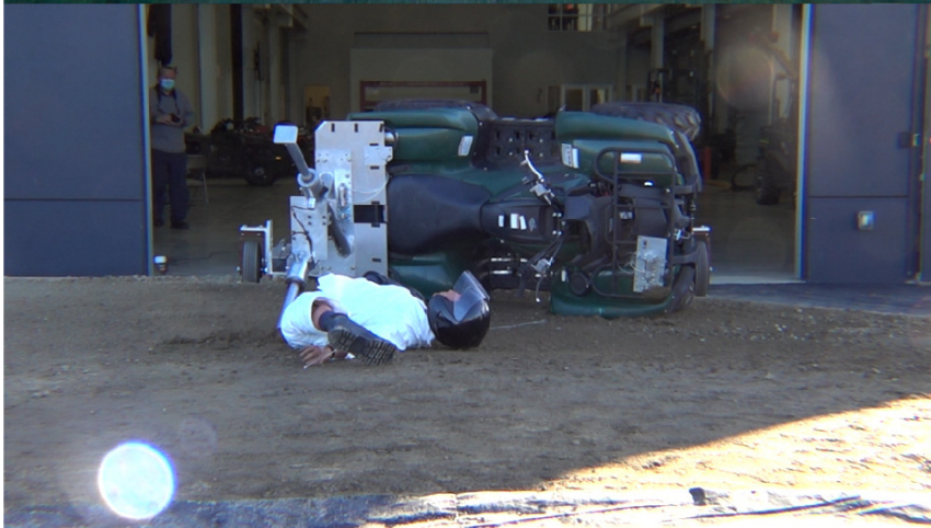
Vehicle C - Sled Moderate Energy Rollover – POC #3 – Extended Span OPD
