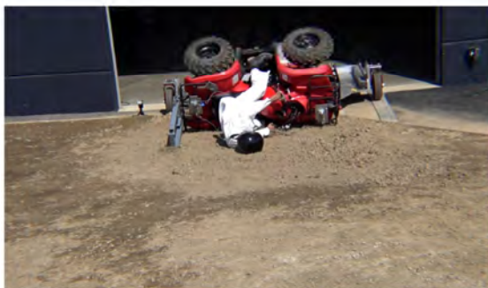
Drone Camera - ATD Head Strike - Time = 0.94 sec
