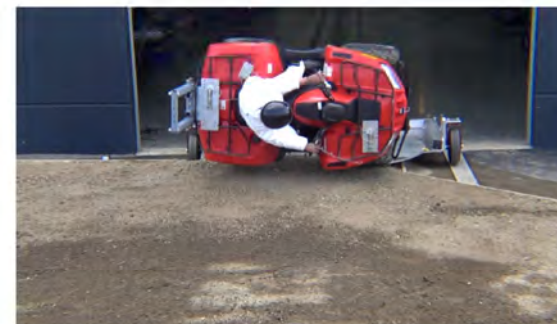
Drone Camera - Roll Angle = 90° - Time = 0.93 sec
